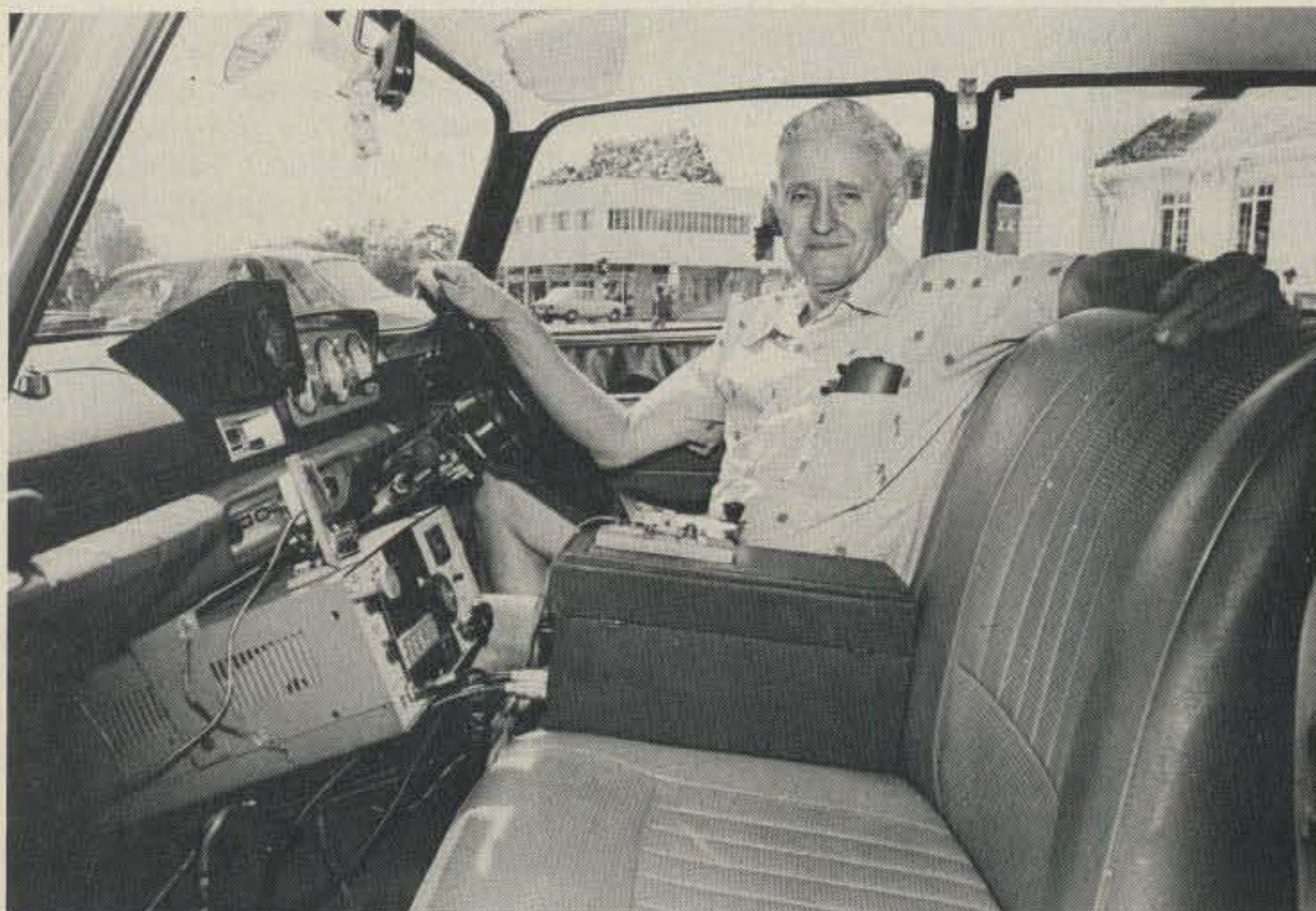
The author seated in the cockpit. The black box houses the impedance matching transformer, spare parts, speaker, and key. The HW-101 has a power meter/s.w.r. bridge on top of it. Up on the dash is an altimeter (we are nearly 5000 feet above sea level). A volt and amp meter to the right measure my power drain.
