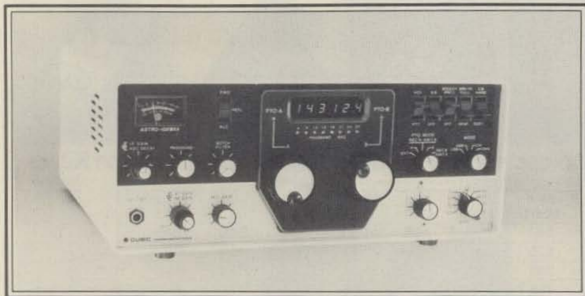
The front view of the Astro-102BXA transceiver. You can follow the passband tuning by the little readouts below the main tuning dial.
