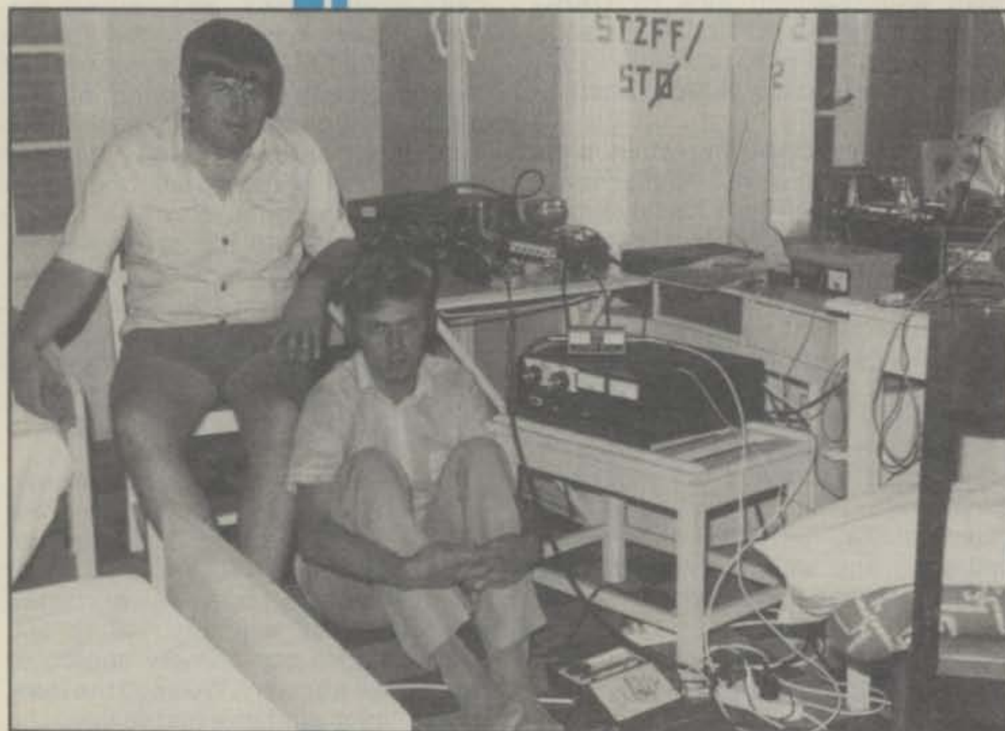
The equipment included a Kenwood TS180 and TS120 with a Dentron linear which were powered by the battery in the middle. The battery was charged when electricity was available.
