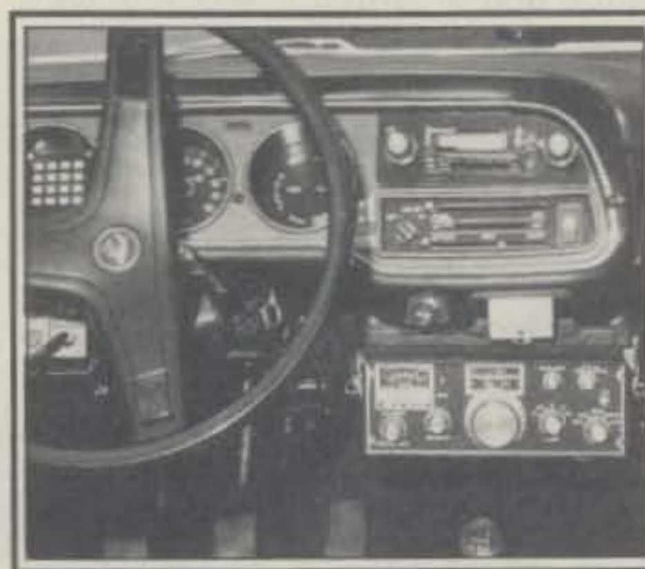
Dash installation showing 2-meter gear, Atlas transceiver and SW broadcast converter.
