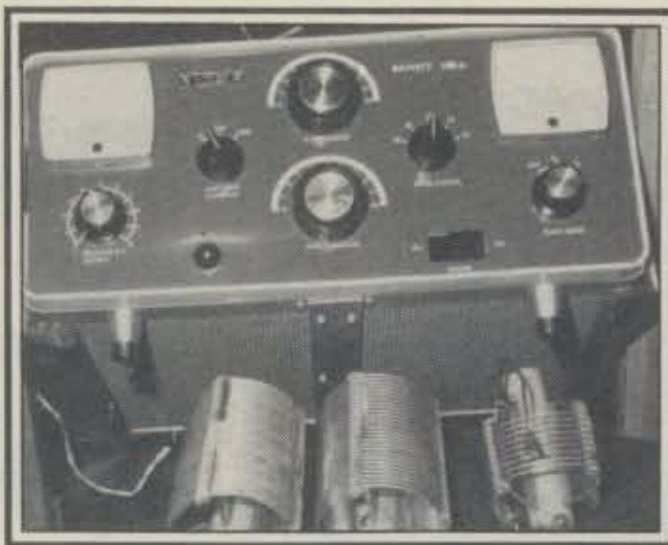
Trunk-mounted linear with antenna coils.
