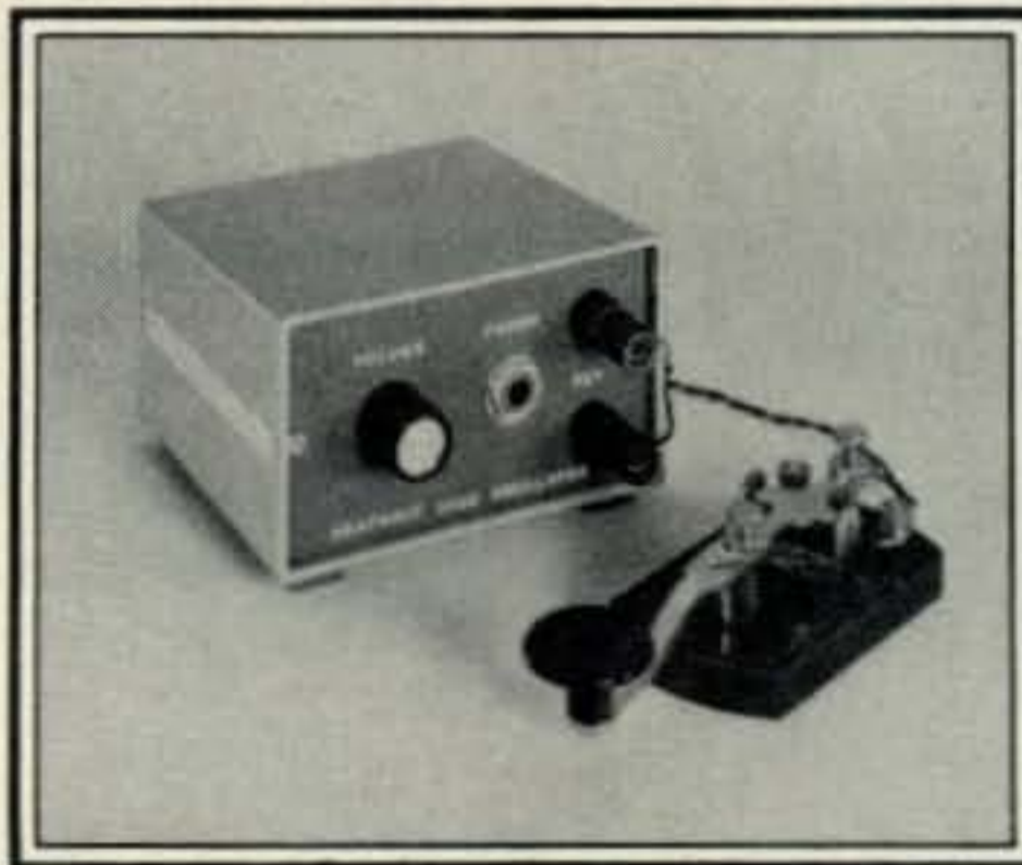
The Heath HD-1416 Code Practice Oscillator before it was converted. It looks basically the same after conversion since it was not necessary to drill any additional holes for controls, etc., in the front panel.
