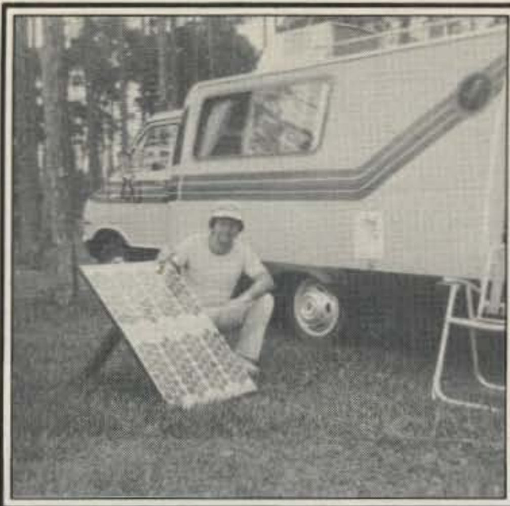
K4KJP displaying his solar array used as the sole power source for 9 QSOs and for charging the nicads used during the remainder of his activity. More fellows should try this approach.
