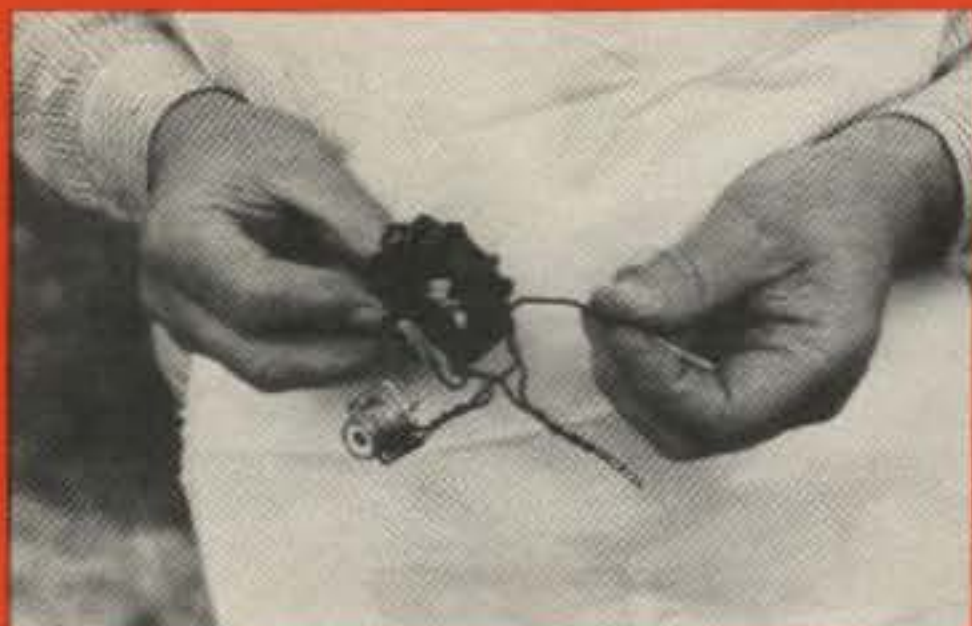
Ferrite-core balun is supplied by the manufacturer in kit form. Unit was easy to make, but it is exposed to the elements with the attendant possibility of inducing erratic matching conditions. A commercial sealed 1:1 balun was later substituted by this reviewer.
