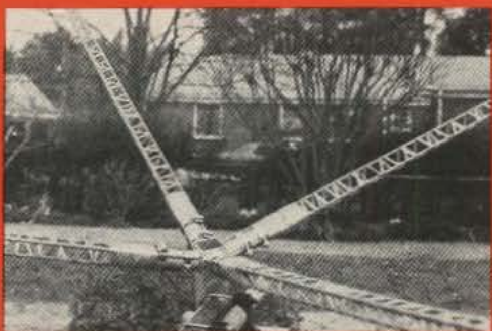
Fiberglass spreaders emanating from the aluminum spider block. Note unusual ribbed or "tridetic" constructions of the arms. Though not a problem in the author's climate, the tridetic design, though extremely rugged, could be vulnerable to ice buildup.
