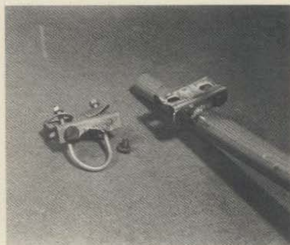
Fig. 1- A \frac{1}{16} " bracket is welded to the boom. This predrilled bracket is screwed to the spreader bracket which has been drilled and tapped.
