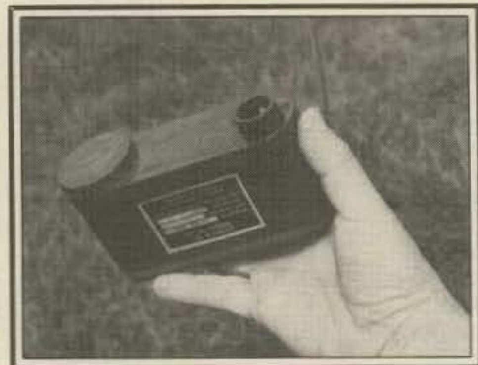
The miniature RC-3A v.h.f. receiver.
