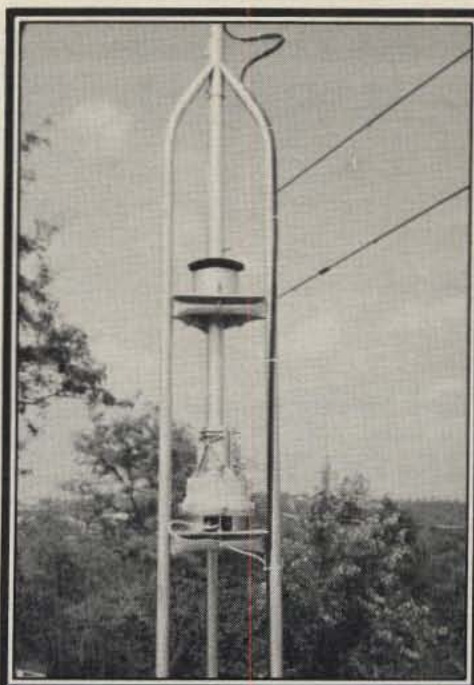
The rotor is shown here with the thrust bearing assembly.
