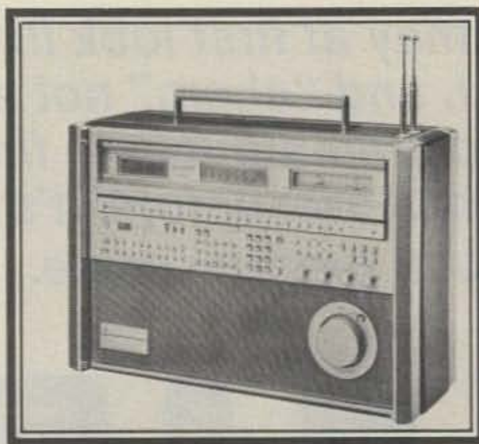
Any shortwave receiver capable of single sideband reception, whether portable (as this digital Panasonic unit) or desk-top, will detect RTTY transmissions.
