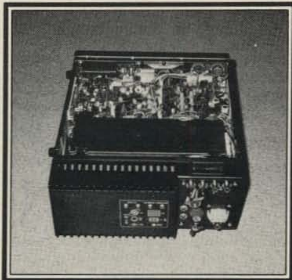
This view shows the IC-720A with the top cover removed. Construction is extremely neat. The view also shows some of the connectors on the back panel and the flat-backed heat sink for the PA.
