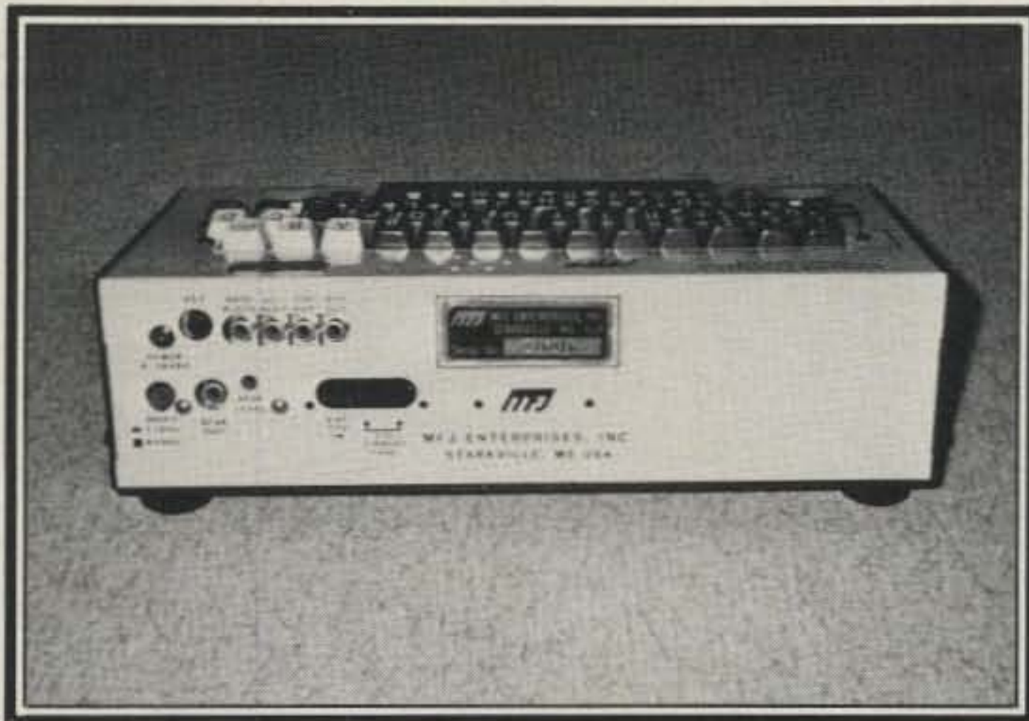
Rear view of a keyboard shows provisions for external connections. The optional TTY Loop module has not been installed, hence the blank hole in that position. All jacks are commonly used, standard-size types.
