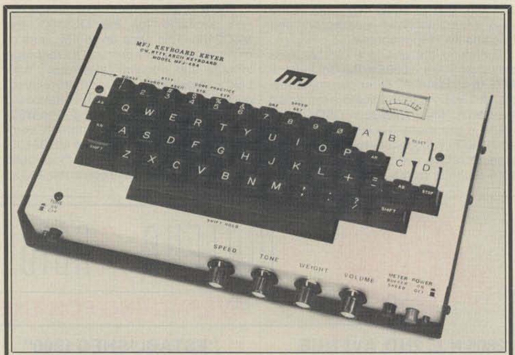
The MFJ-494 and MFJ-496 keyboards are completely self-contained with all the electronics, including optional equipment, housed inside the cabinet shown. Latter models also include various colored keys for certain functions which makes command entries easier to remember.
