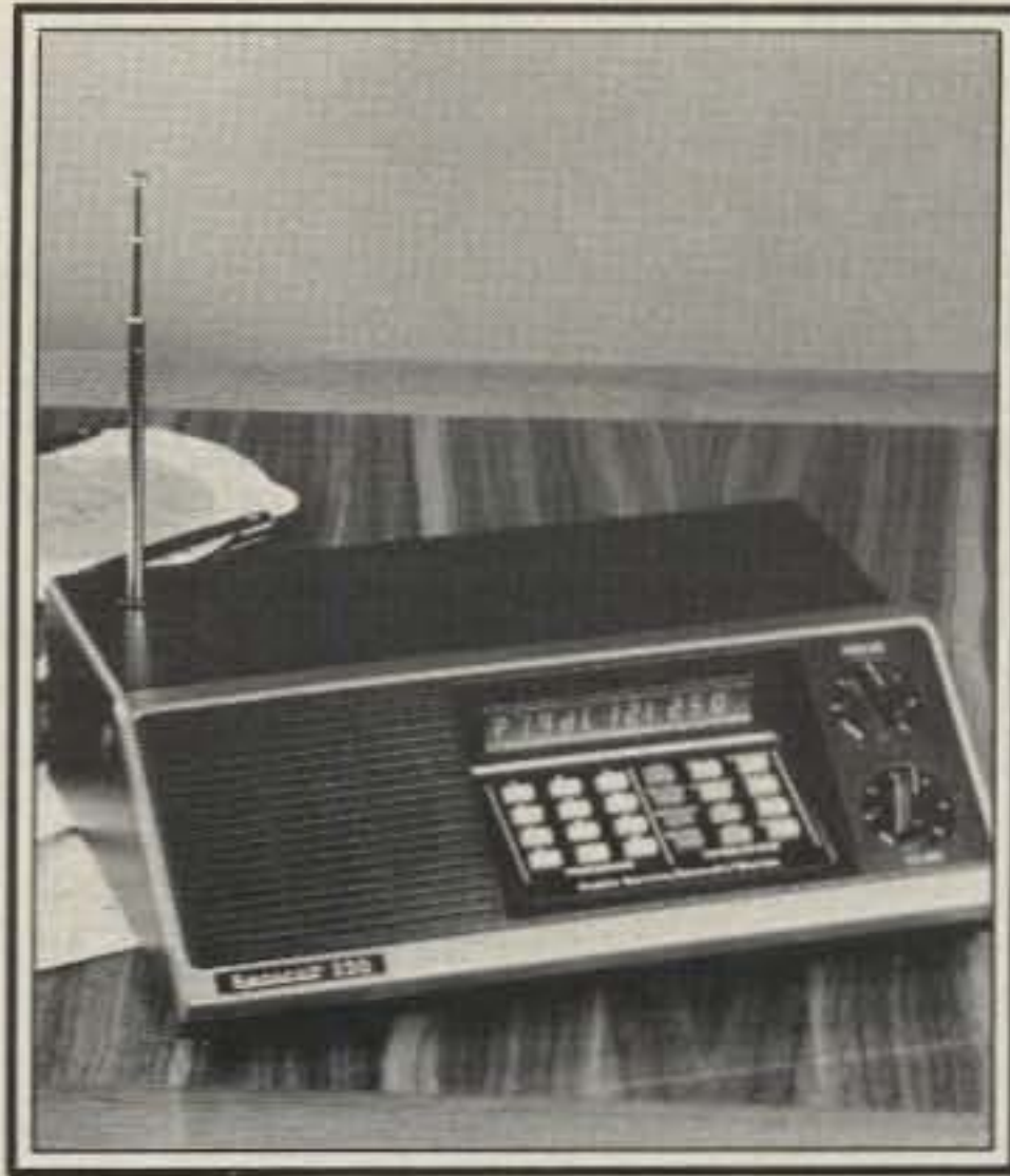
For the sophisticated s.w.l. who wants to roam the higher frequency ranges, the Bearcat 220, shown here, allows monitoring of all the public service ranges plus the a.m. aircraft band. Up to 20 frequencies may be scanned at the same time. In addition to "normal" scanner functions, where frequency limits are set and the scanner searches between programmed parameters, it also searches marine or aircraft frequencies by depressing a single button. These frequencies are stored in memory, so no reprogramming is required. Other state-of-the-art features include priority channel and dual scanning speeds. (Photo courtesy Electra Co., div. of Masco Corp. of Indiana)
