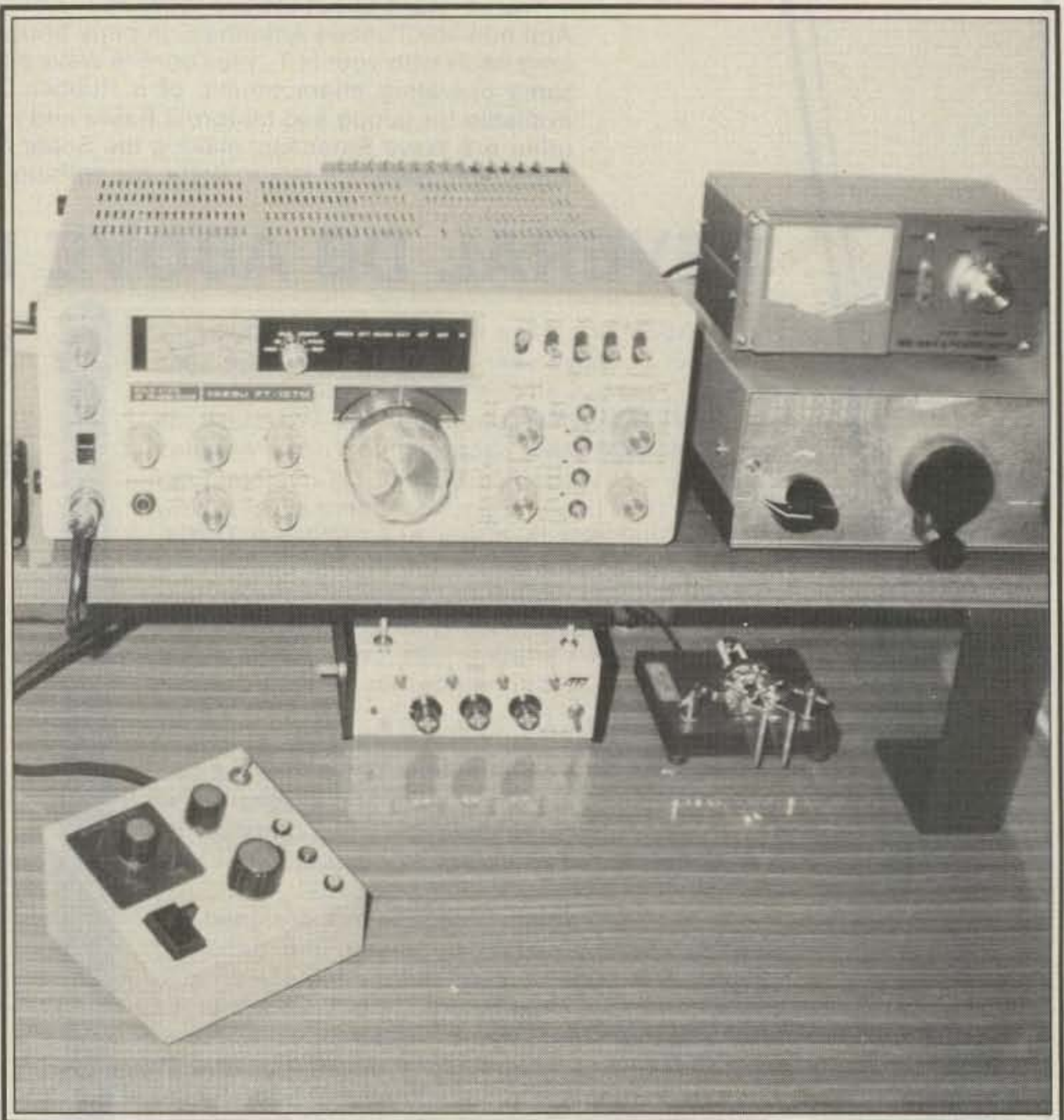
The tune-up circuitry described is housed in the small control box shown in the foreground. The control box also has some other handy features as mentioned in the text.
