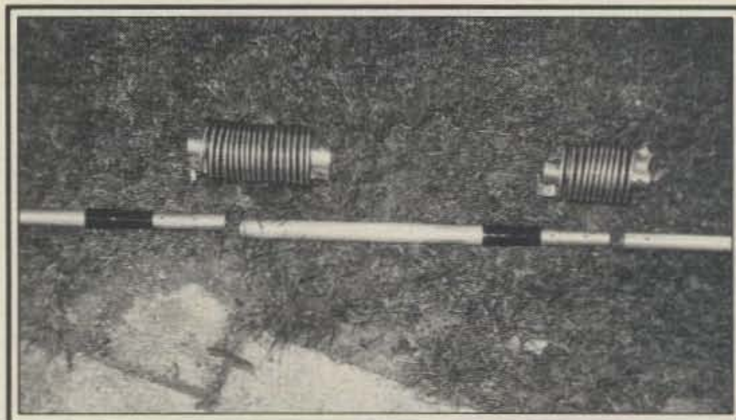
The 80 and 40 meter resonator coils. When the tubing sections are joined, the coils will straddle the insulating section on each tubing section.
