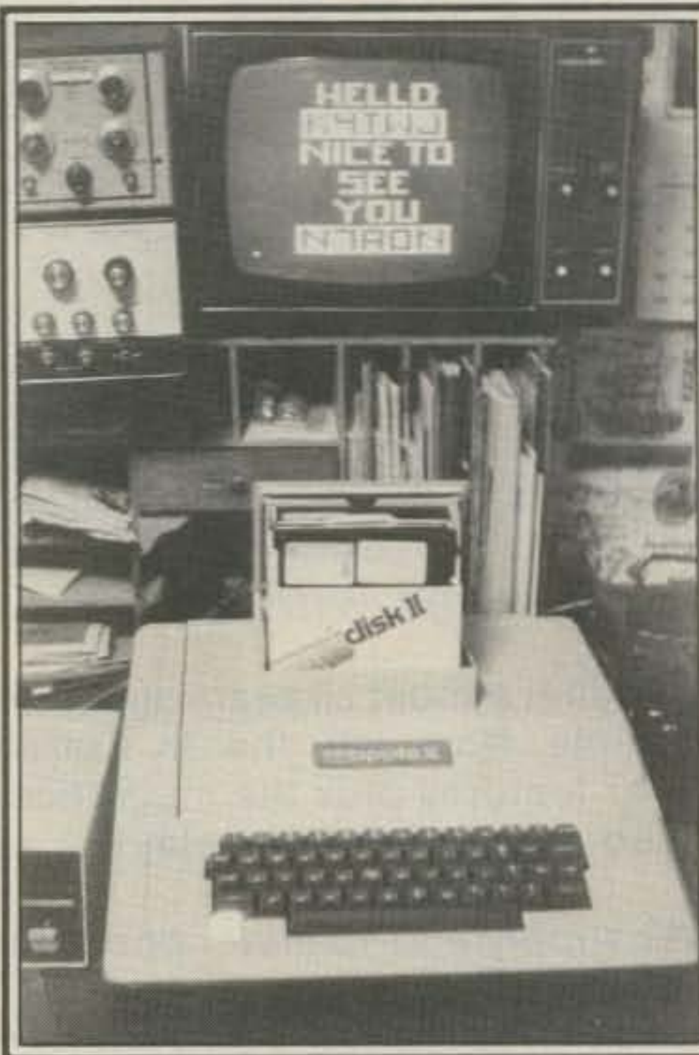
The N7AON SSTV keyboard/titling system which loads an Apple II via disc provides several unique functions, including "canned" messages with "fill-in" blanks. A two-punch keyboard action brings up those programs.
