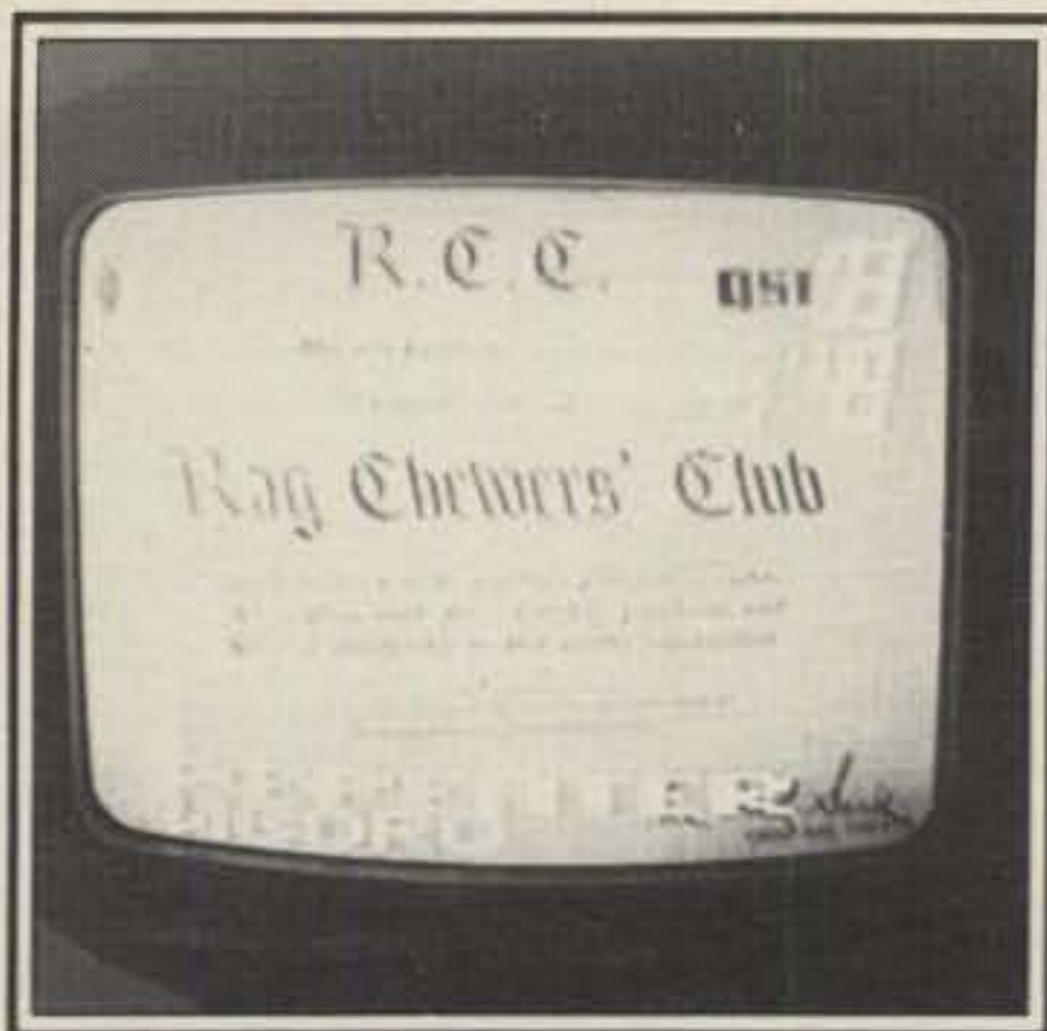
Here's W6ORG's video "returning" through his crossband FSTV machine described in column. The "93" in right top is repeater's a.g.c. level superimposed on video. Below that is Time Display also superimposed. Repeater ID is at bottom.
