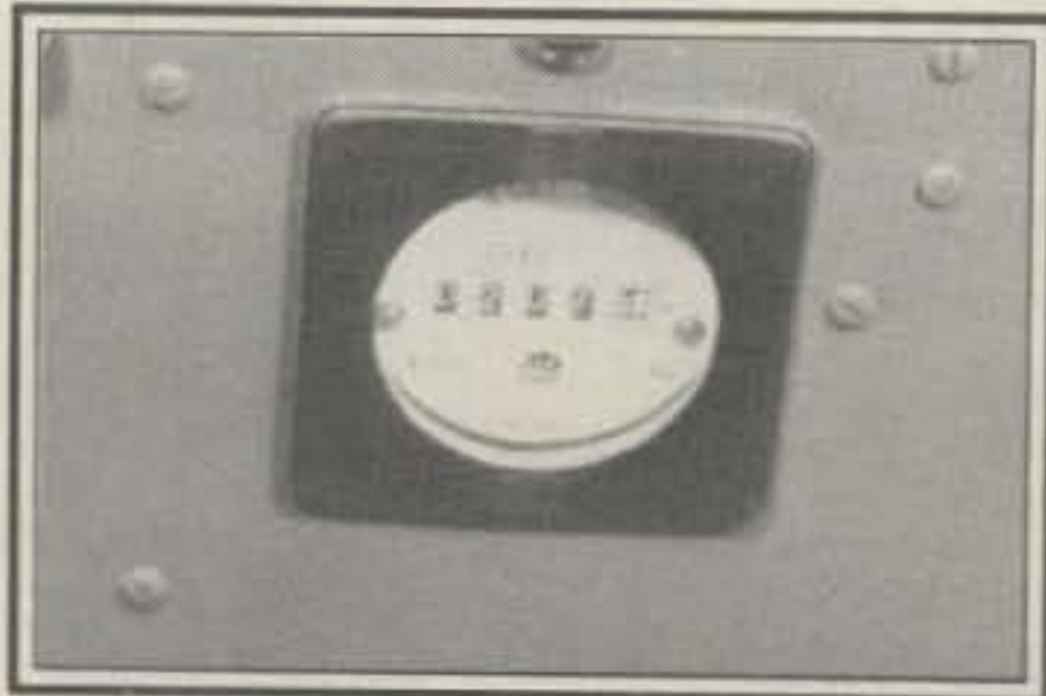
Here is that running time meter we mentioned in the text. Since then, there is a lot more time on the supply.
