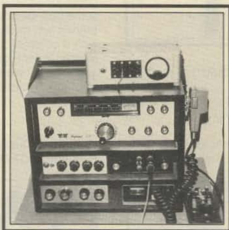
The author's small-power small-size station, including threshold limiter, notch filter, speech processor, a.t.u., and 2-meter transverter, with external power supply at top.
