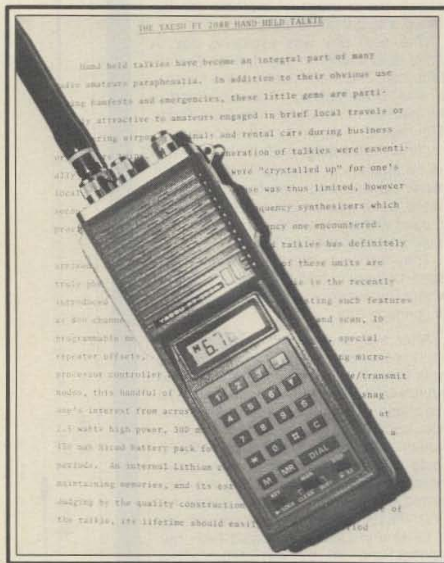
The Yaesu FT-208R 2 meter HT shown across the first page of this review's manuscript.
