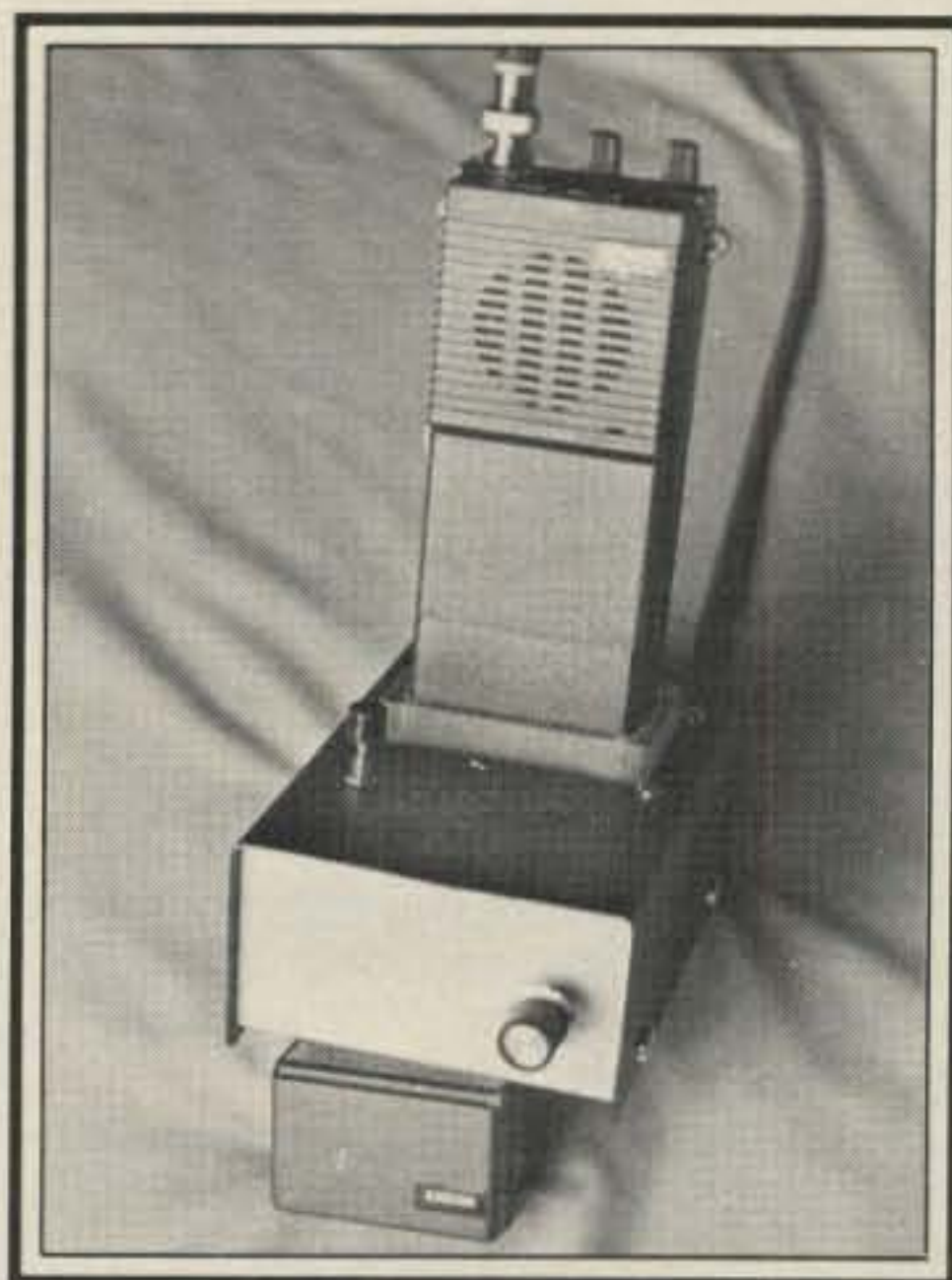
This is the finished charger. The IC-2A has the BP-5 battery pack installed, while the BP-3 is shown below the charger.
