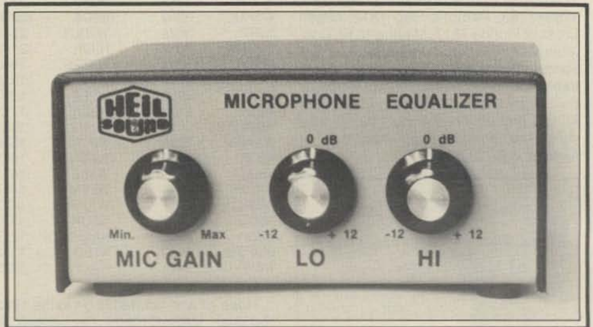
The EQ-200 is housed in a shielded metal enclosure and requires a 9 volt internally mounted battery for power. The jacks for microphone input/output as well as the on/off switch are on the rear panel.
