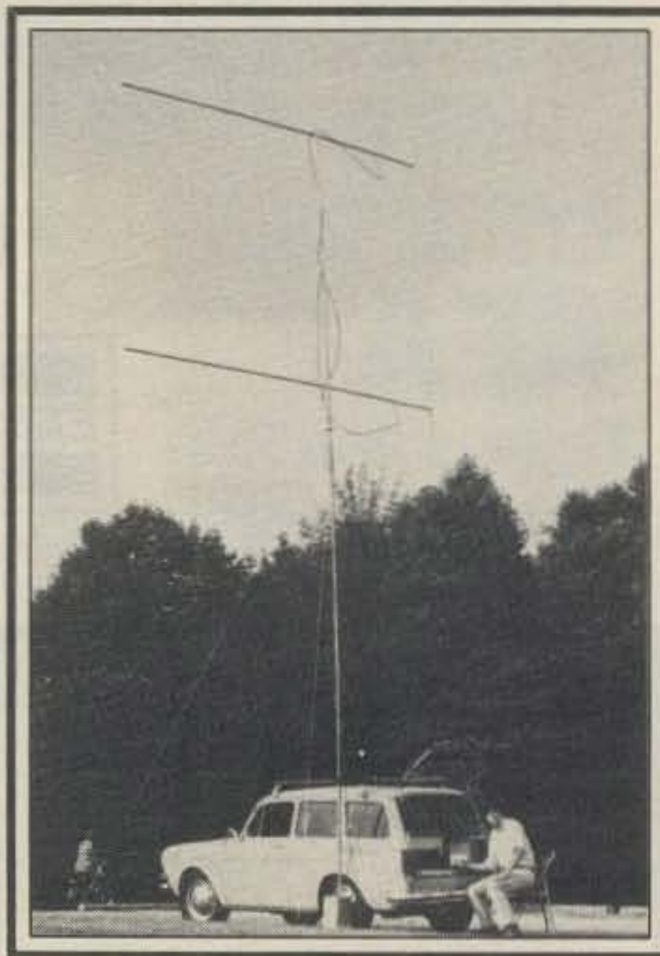
Emil, W3EP, and his mountaintopping setup. The rig is a Yaesu FT-221 and a solid state amplifier. The antenna system is two 8-element quagis. Emil most often uses only one quagi, a system which takes only a few minutes to set up.
