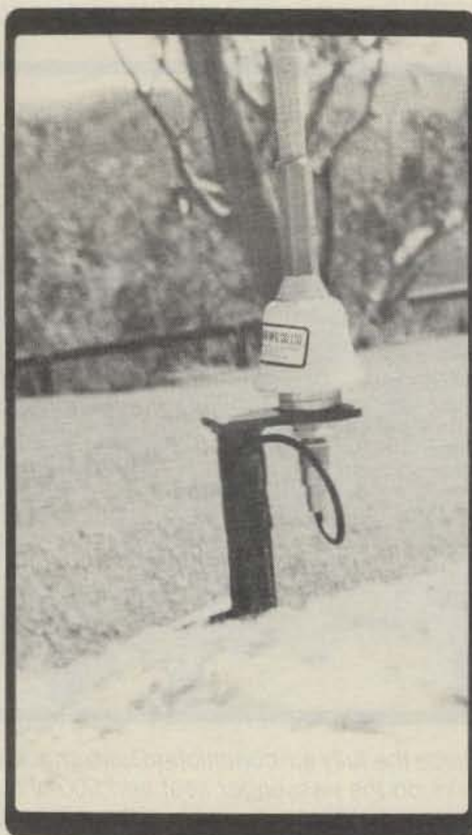
Photo of the mobile antenna bases used. They were designed and built in New Zealand by ZL3RJ. Note the simplicity of mounting and feeding coax to the base. The aluminum whip section terminates into a brass base machined and threaded to fit the antenna base.
