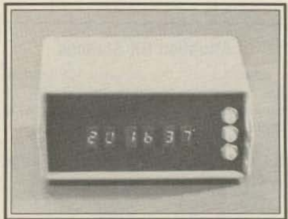
The Hal-Tronix 5314 clock in a Radio Shack 270-218 cabinet. Switches at right are for setting the time. Top button is hold, middle button is slow speed, and bottom button is fast.
