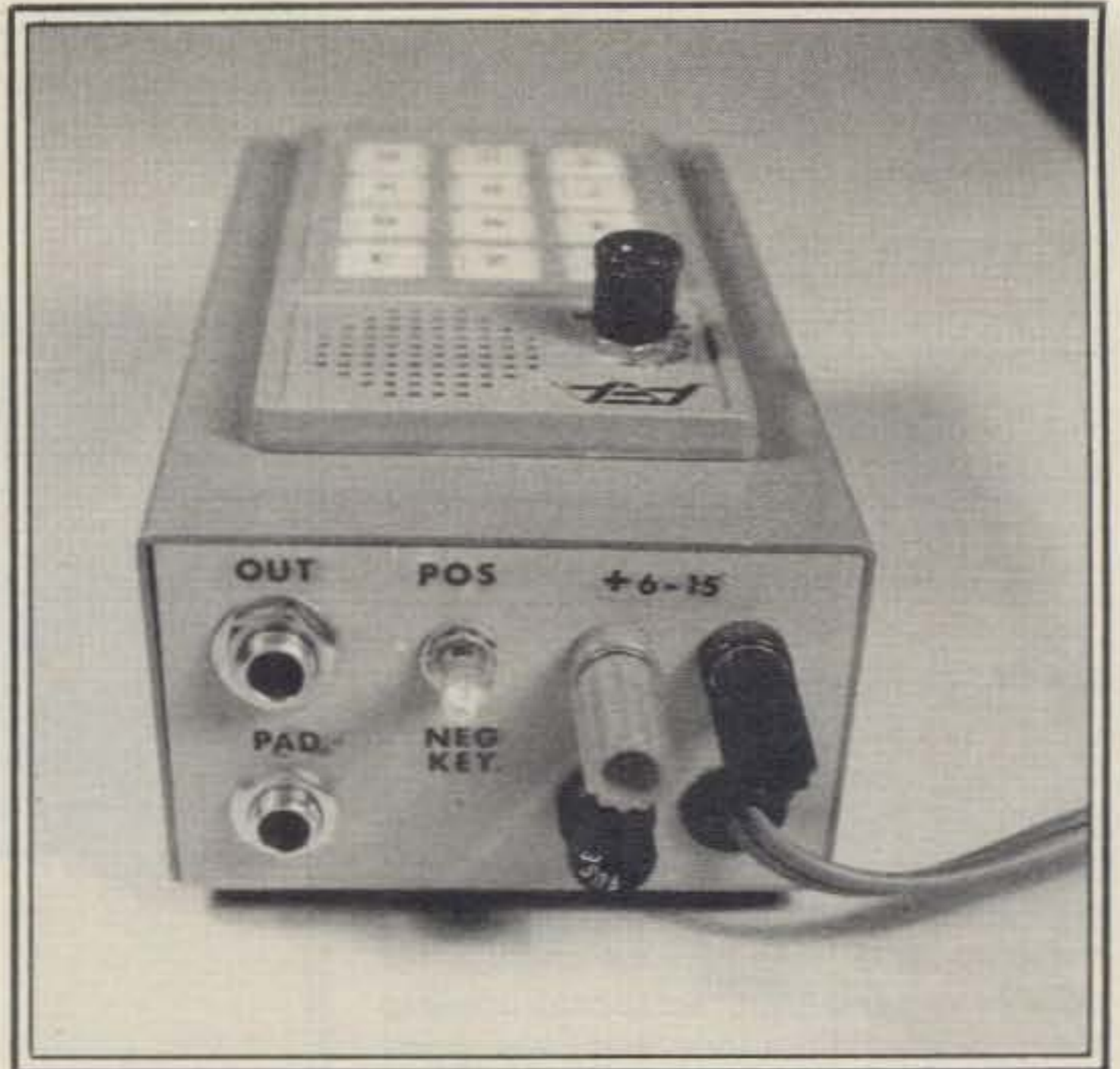
Rear view showing paddle input and keyer output jacks, keying polarity switch S-4, battery binding posts, fuse, a.c. cord.
