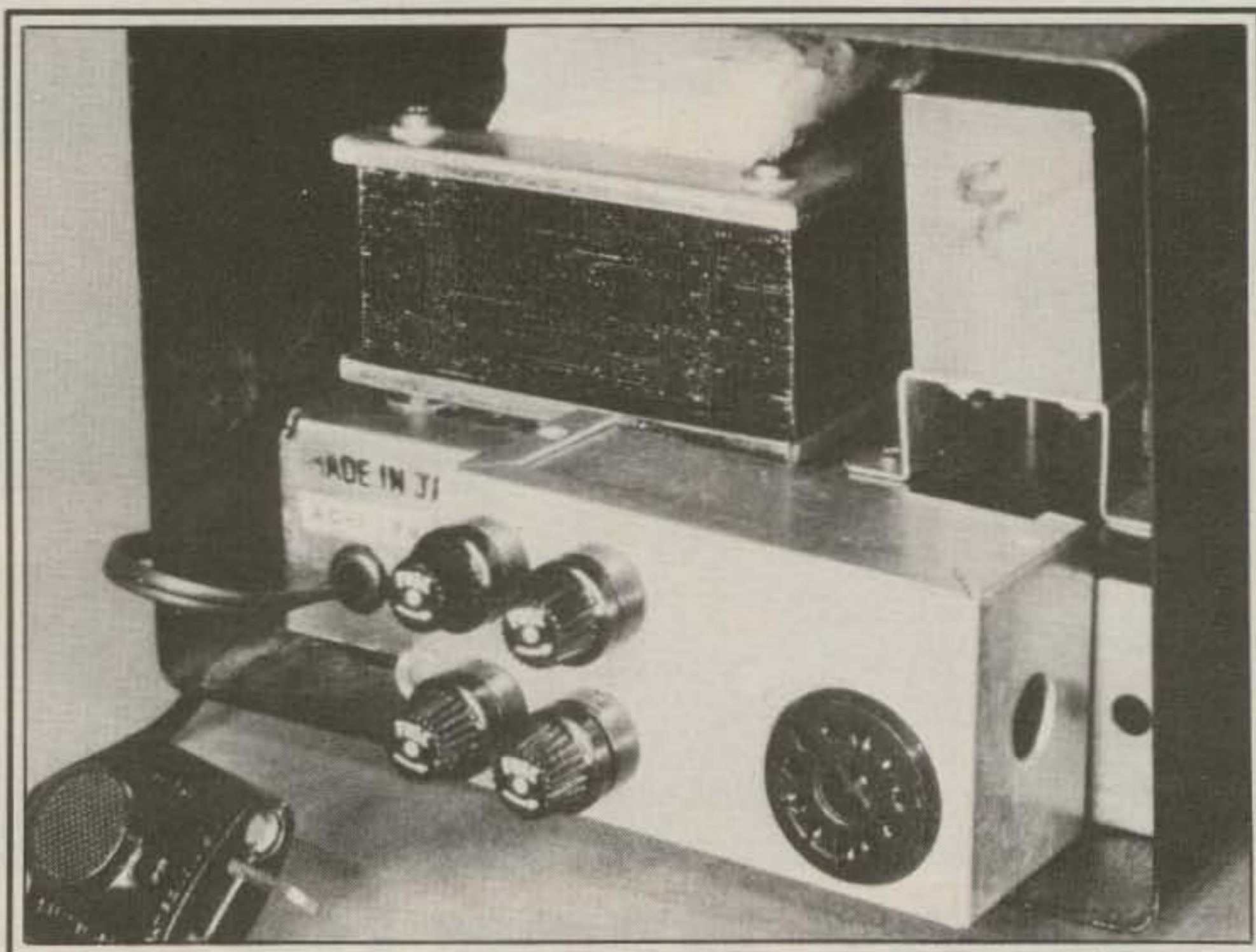
A rear view of my Tempo power supply showing the superfuse riding piggyback on the power output connector. The fuse holders are marked as to amperage and circuit fused. Also note the fused a.c. plug, which was added as a simple means for fusing each side of the input line. (W1GSL photo)
