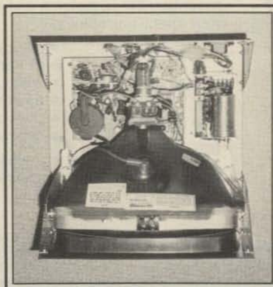
A look inside the ESM-914 video monitor. The a.c. supply is on the right, and the rest of the circuitry is on a large PC board.
