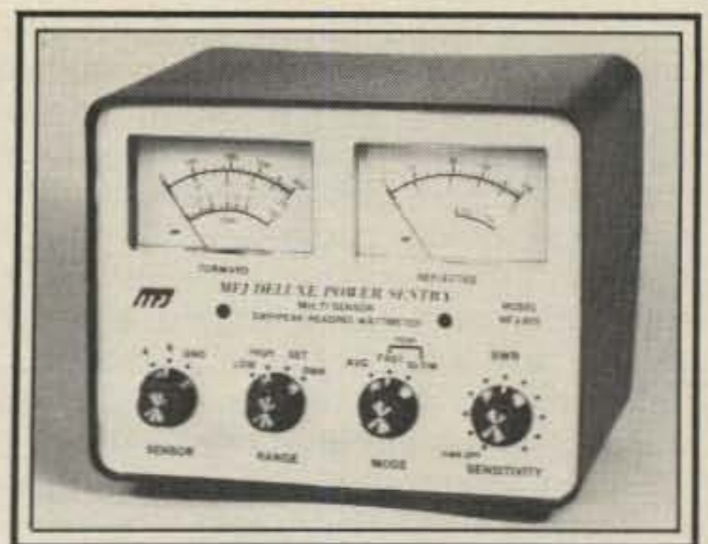
MFJ Model 825 illustrated here is a flexible, multi-sensor s.w.r./peak reading wattmeter for h.f., v.h.f., or QRP transmitters and transceivers. The three specialized sensors can be plugged in simultaneously; a front-panel switch selects which rig to monitor. H.f. sensor handles 2000 watts to 30 MHz; v.h.f. sensor handles 200 watts to 175 MHz. QRP sensor is for 20-watt (or less) operation to 30 MHz. (Photo courtesy MFJ Enterprises, Inc.)
