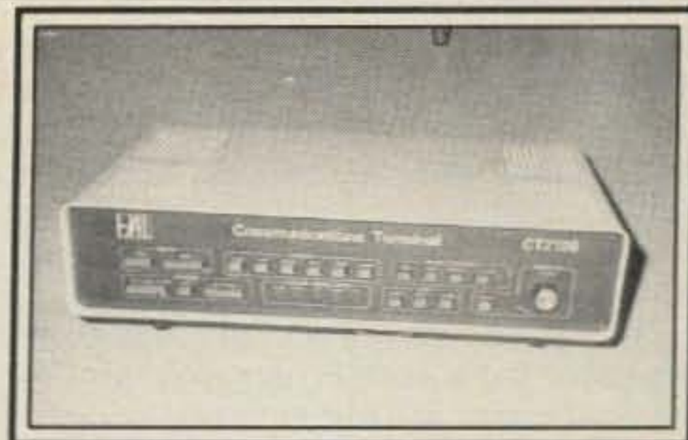
The heart of the system is the CT-2100 communications terminal. It measures about 16½" x 4" x 10½".
