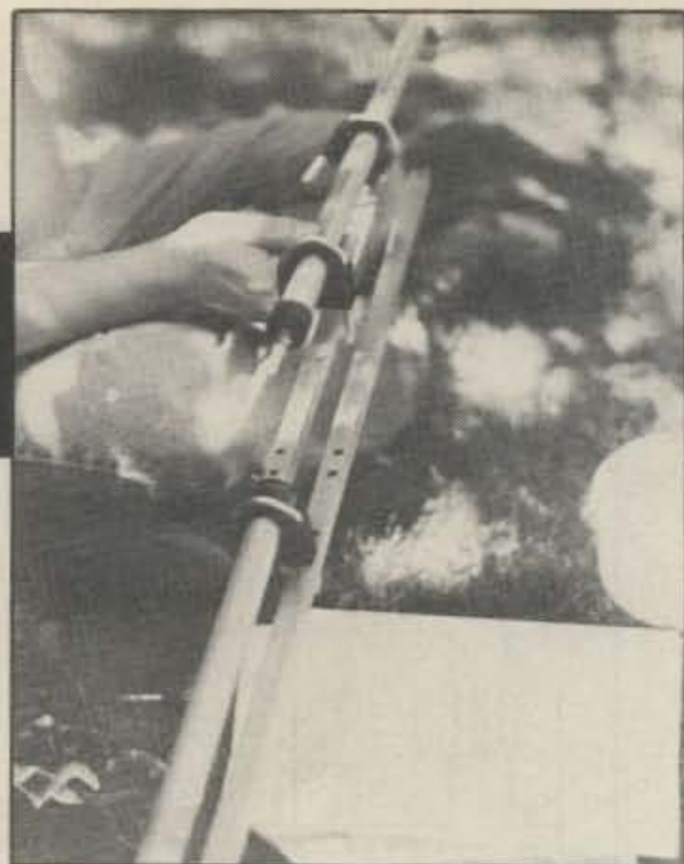
Close-up of a typical radiator/reflector assembly.
