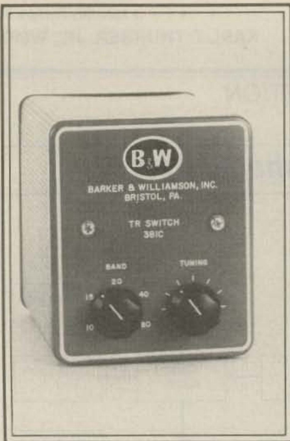
Electronic antenna changeover switch has no moving parts. In this B&W model, the transmitter is continuously connected to the antenna, while the antenna circuit to the receiver is blocked during transmit. Switching is virtually instantaneous for fast break-in operation. Unit handles 2 kw PEP and has a built-in receiver preamplifier. (Photo courtesy Barker and Williamson)
