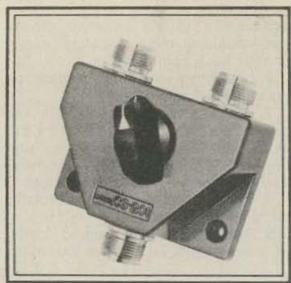
Simple and straightforward Daiwa coaxial switch is designed for operation to 500 MHz and particularly suitable for switching between two antennas or two transceivers. The s.p.d.t. switch is of the type that automatically grounds the unused terminal. (Photo courtesy J.W. Miller div. of Bell Industries)
