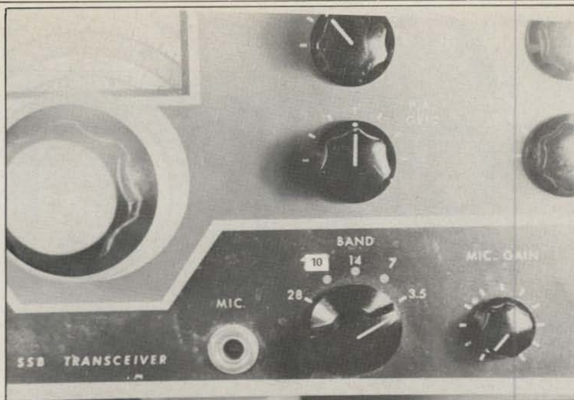
Front view of the modified Swan 350C. The 21 position has been changed to 10.
