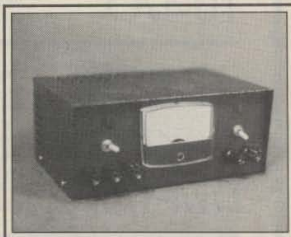
The workbench LV power supply.
