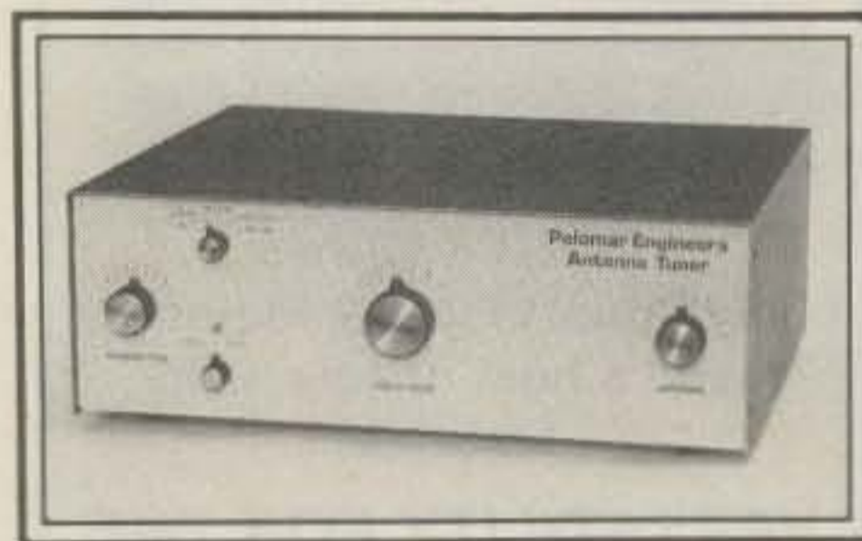
There is no reason why the antenna noise bridge can't be teamed up with an antenna tuner in a single package for tune-up without the need to apply transmitter power. The Palomar Engineers PT-3000 tuner shown here allows tune-up without going on the air, yet the built-in ANB lets the operator preset the tuner for a 1:1 s.w.r. without reference to the transmitter. Unit is designed for continuous coverage, 1.8–30 MHz, with a power rating of 2000 watts; coax, single-wire, and balanced-line antennas can be accommodated. A source of 9 v.d.c. at 50 ma is required in the tuneup mode. Although in the $400 price class and designed for high-power operation, this type of antenna tuner would likely be of interest to the serious shortwave listener, due to the precision antenna matching possible with such a combo. (Photo courtesy Palomar Engineers)
