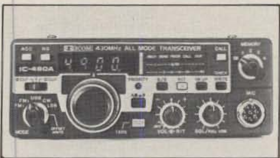
Here's ICOM's recently introduced IC-490A, an all-mode, 10 watt transceiver covering 430 to 440 MHz. The unit can be used for receiving OSCAR 8 mode "J," and when combined with a 50 or 100 watt amplifier and 10 dB gain antenna, will provide a good uplink signal for OSCAR Phase III mode B. Another Phase III capability, mode "L," can also be received on 435 MHz.
