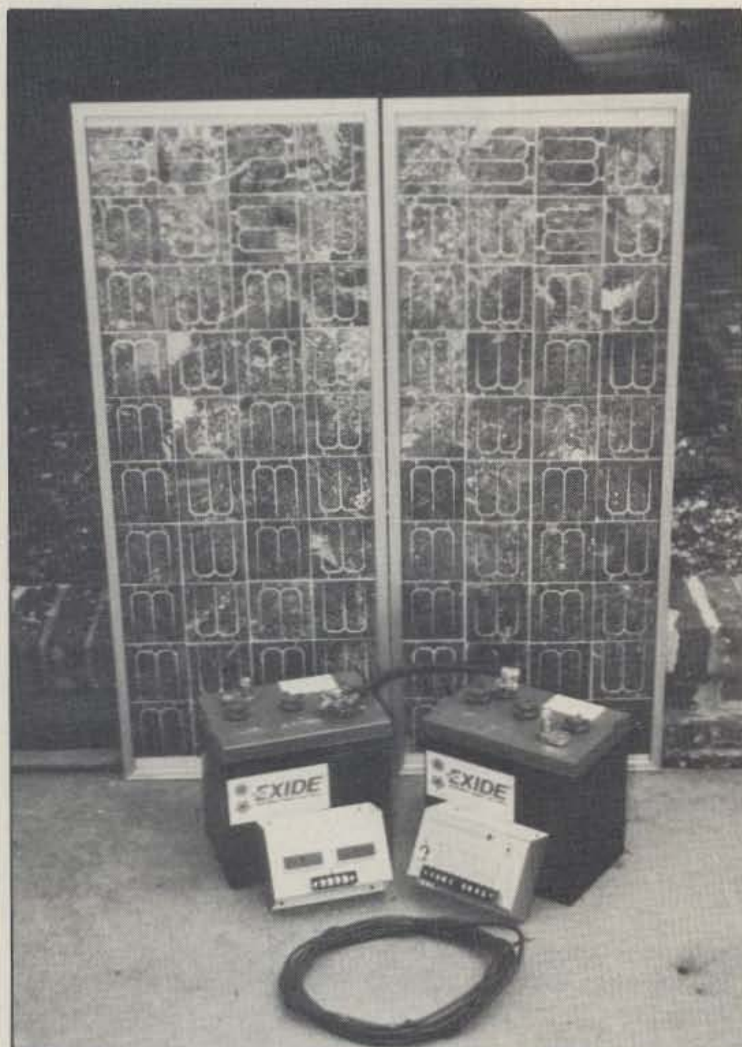
This is the system described in the review. The solar panels are shown, and in front of them are the batteries, metering box, and sun-charger unit.
