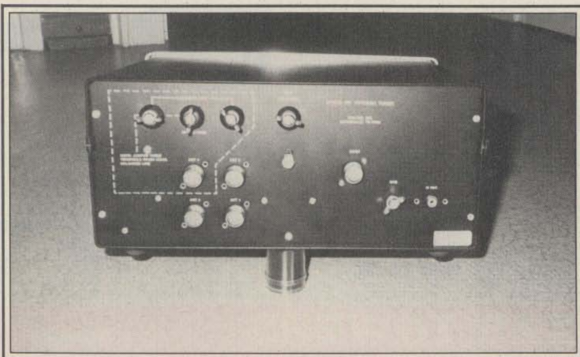
The back panel of the 229 is nicely arranged with the various output connectors for coaxial lines, single-wire antenna, and balanced transmission line on the left with input, ground, and dial lamp power connectors on the right.
