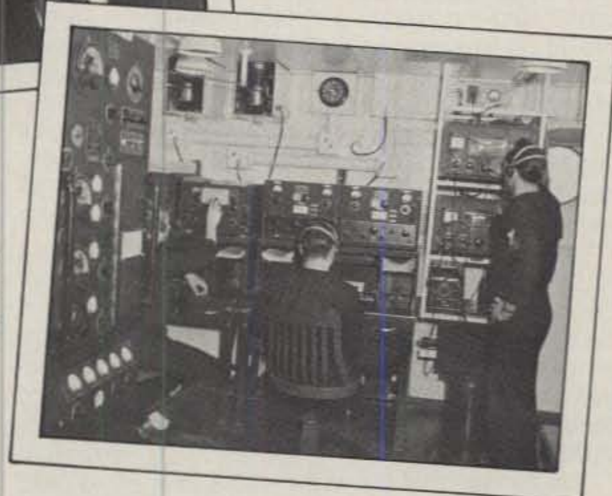
Radio room aboard ship in World War II. One kilowatt transmitter (left) and receivers (center and right). (Official U.S. Navy photograph.)
