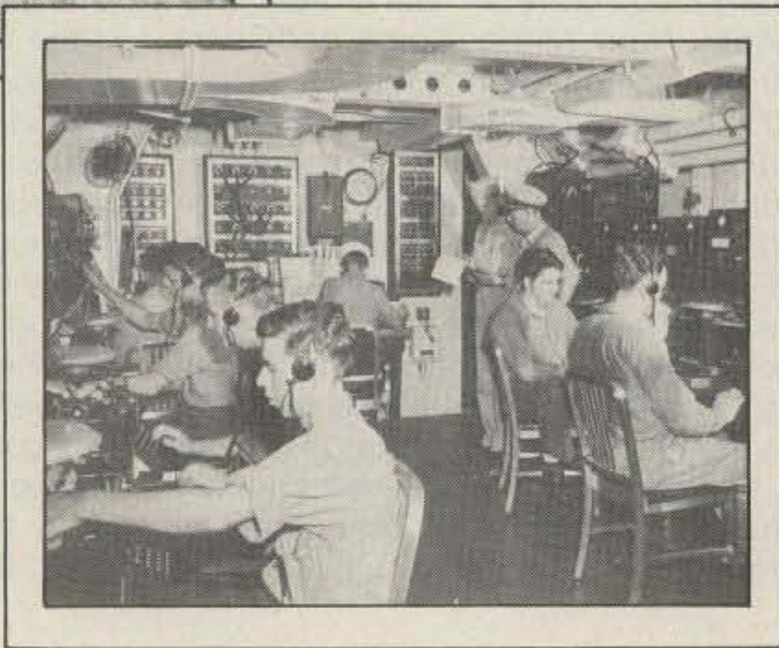
Radio Central aboard a cruiser in World War II. All copy is on typewriters. Transmitters were located in a separate compartment. (Official U.S. Navy photograph.)
