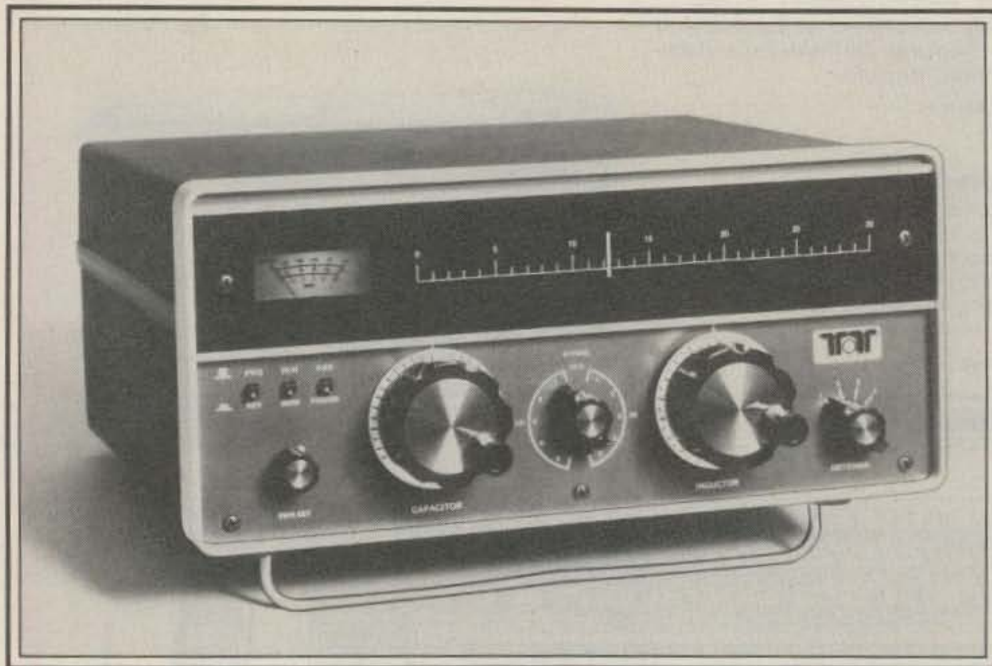
The Model 229 is a smartly styled unit. Two large tuning knobs are used for the variable capacitor and variable inductor elements, while a linear dial scale (0-30) indicates the turns setting for the inductor.
