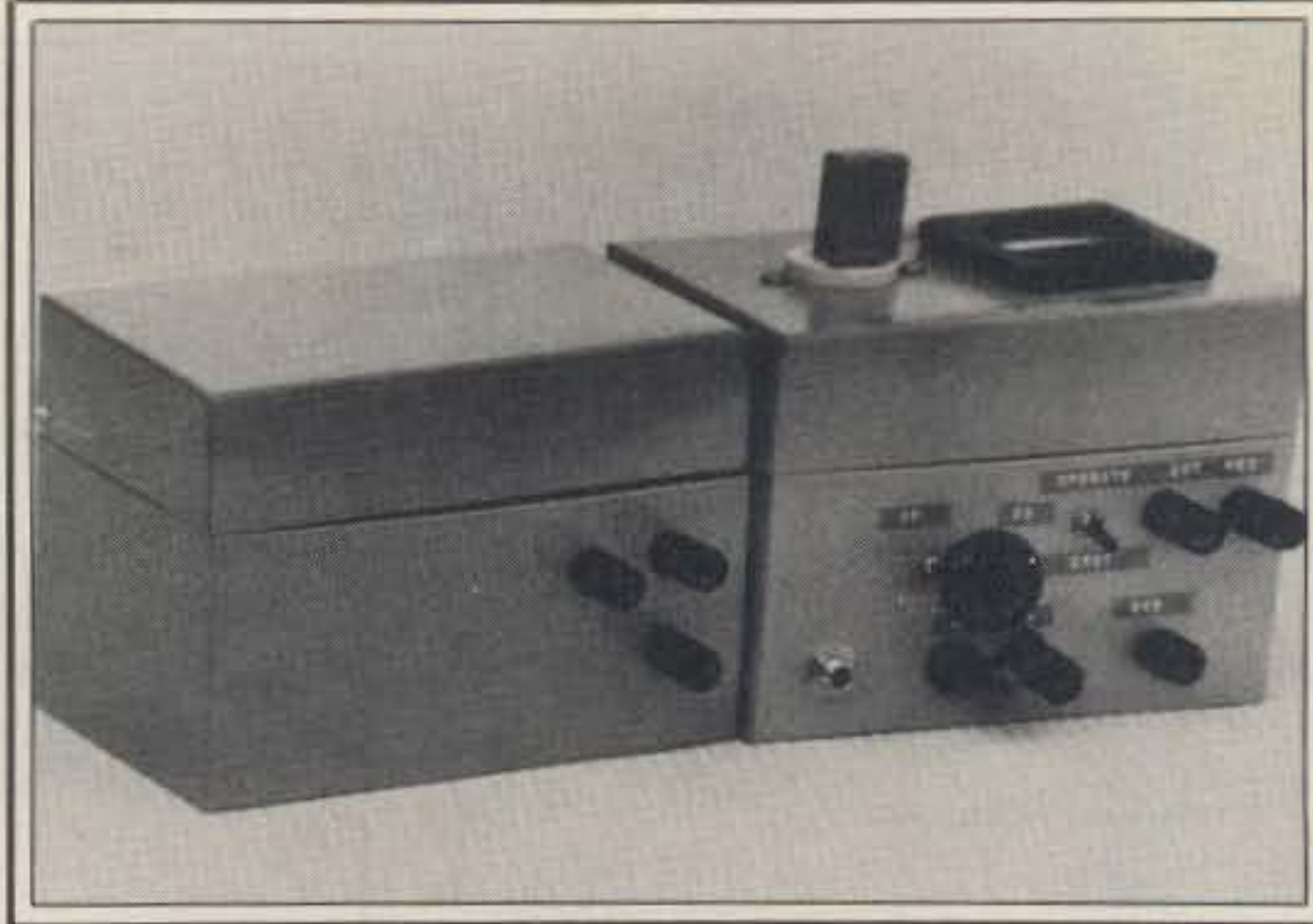
Transmitter with matching power supply; fuse is inside box.
