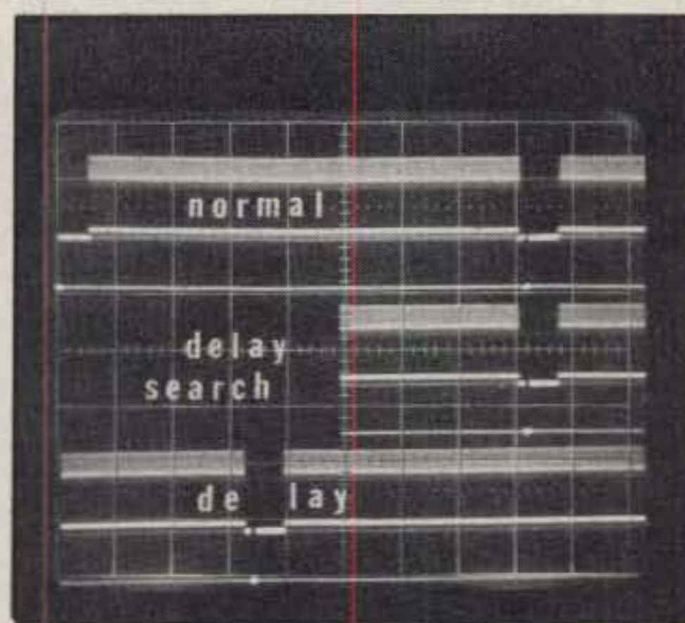
Fig. 2—One waveform seen in the normal, delay search, and delay positions.
