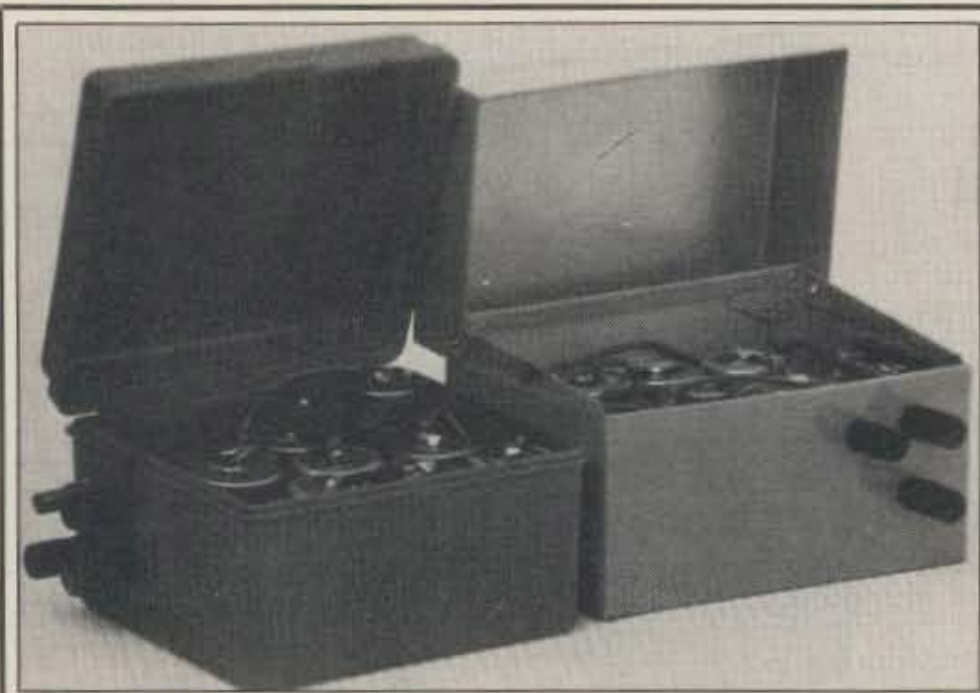
Two battery packs are for added power, about 26 volts total. The extra binding post has a diode series connected to aid in recharging the batteries.
