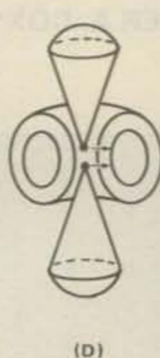
Fig. 4- Evolution of sleeve-dipole antennas from sleeve-monopole antennas.
