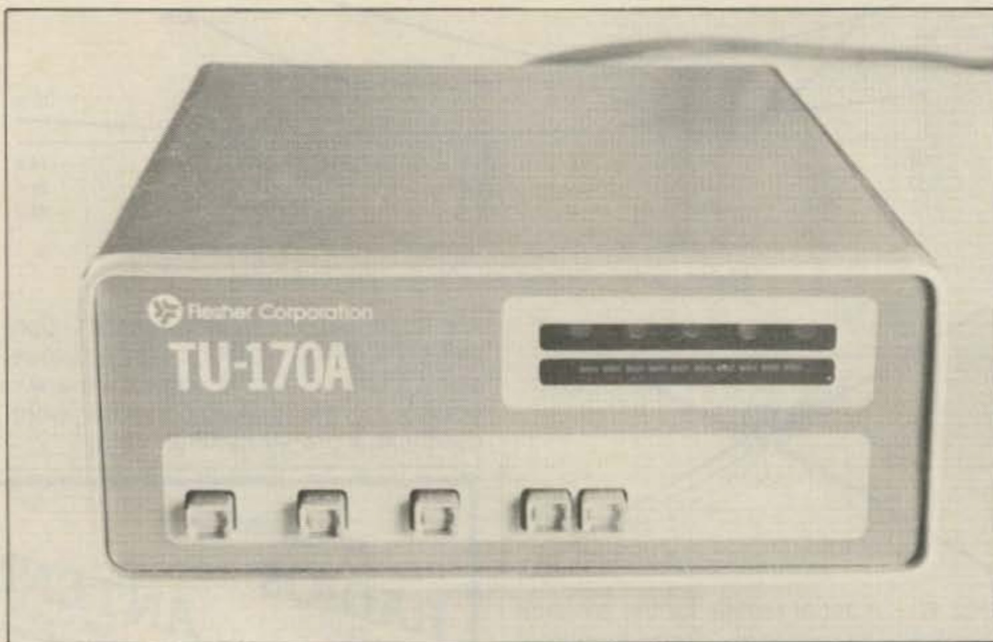
This is a front-panel view of the TU-170A. At bottom left is the power switch, followed by the standby/operate, the send/receive, the reverse send, and reverse receive switches. At the upper right are the LED indicators described in the text.
