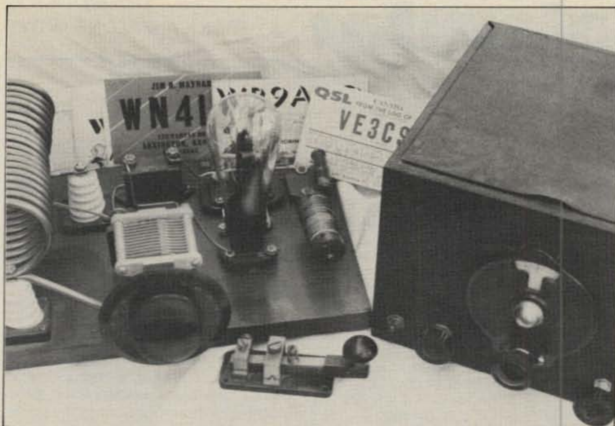
Classic amateur gear from the 1930s can be refurbished and used on c.w. for many exciting QSO's. Rig shown here is number 10 tube transmitter, vintage key, and National SW-3 receiver. Rig has turned many 80 meter contacts at K4TWJ.
