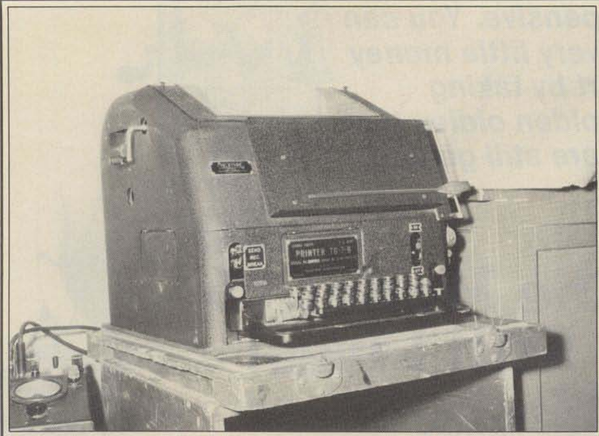
The TG-7B, the military version of the Model 15 teleprinter.
