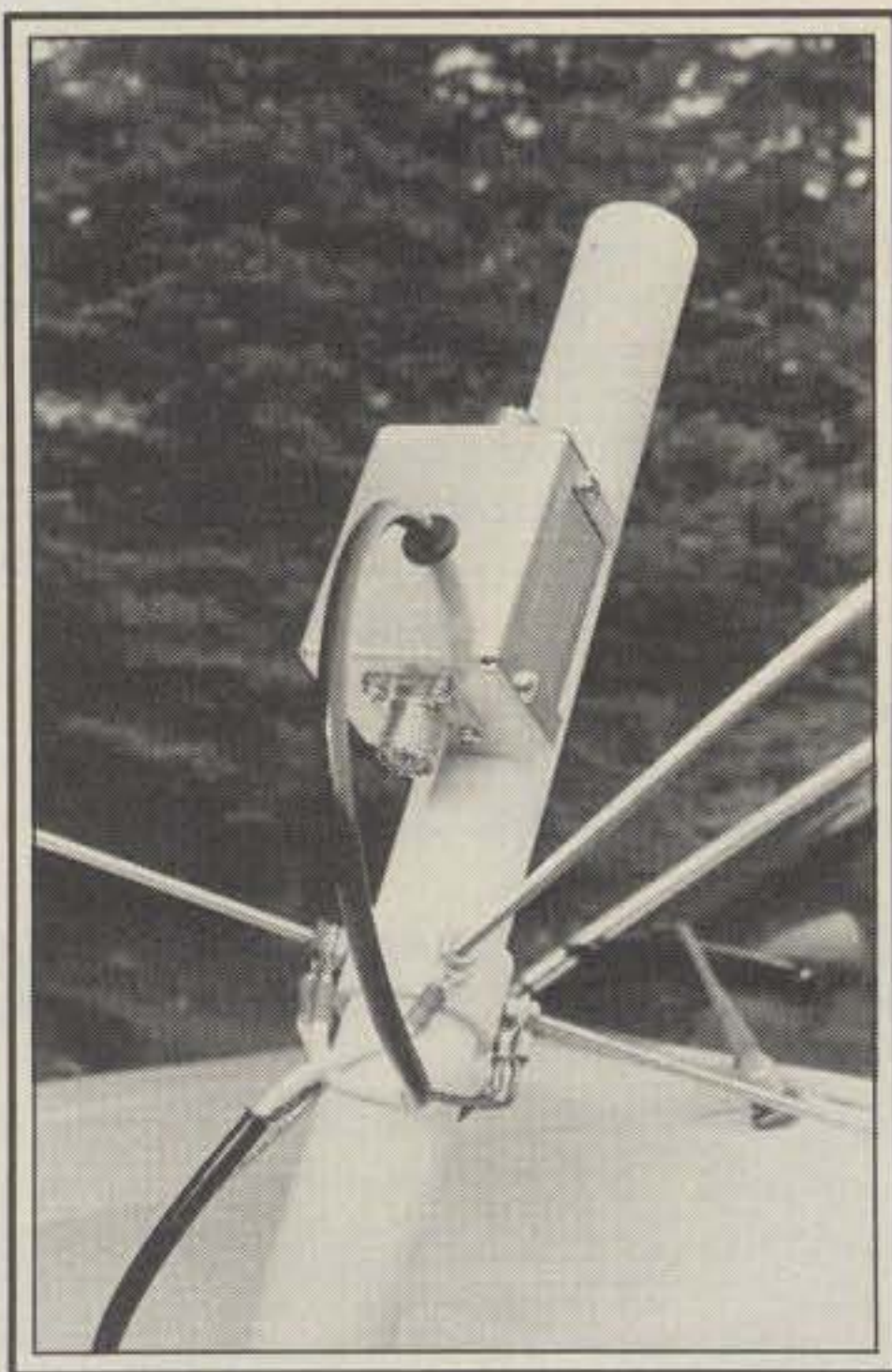
Close-up view of the 8-32 threaded rod assembly. The four rods are cut to 20 inches and then trimmed back via fine tuning. Make sure that the four rods do not make contact within the PVC and internal dowelling.
