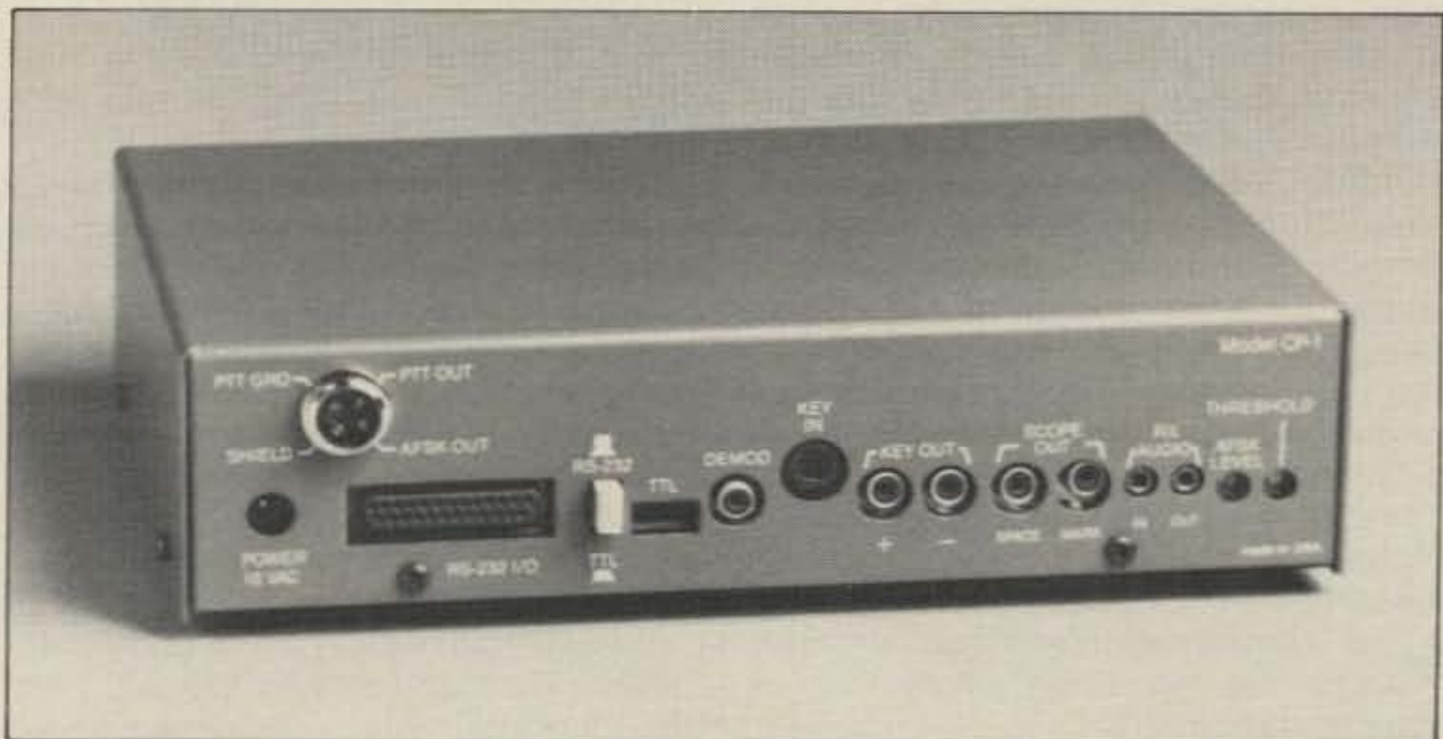
Rear connections on the AEA CP-1 permit quick and easy interfacing with a variety of amateur gear.
