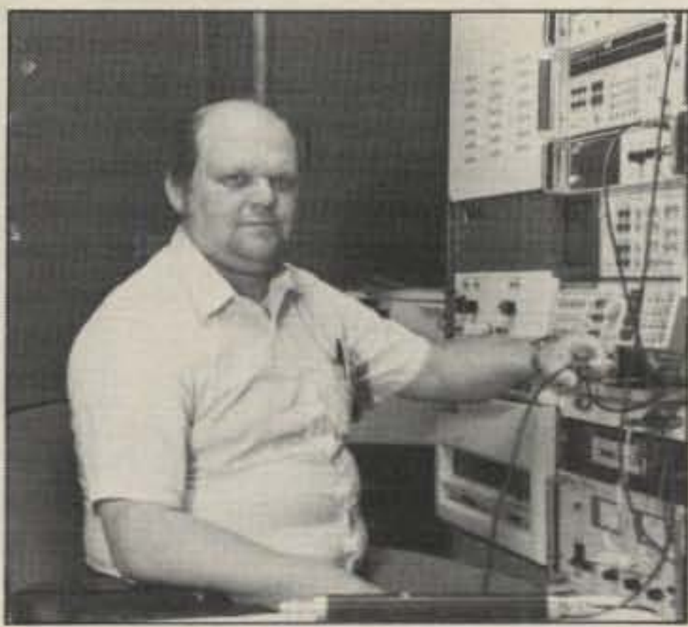
Engineer Dan Stanks uses a spectrum analyzer to measure the response of an interference filter.
