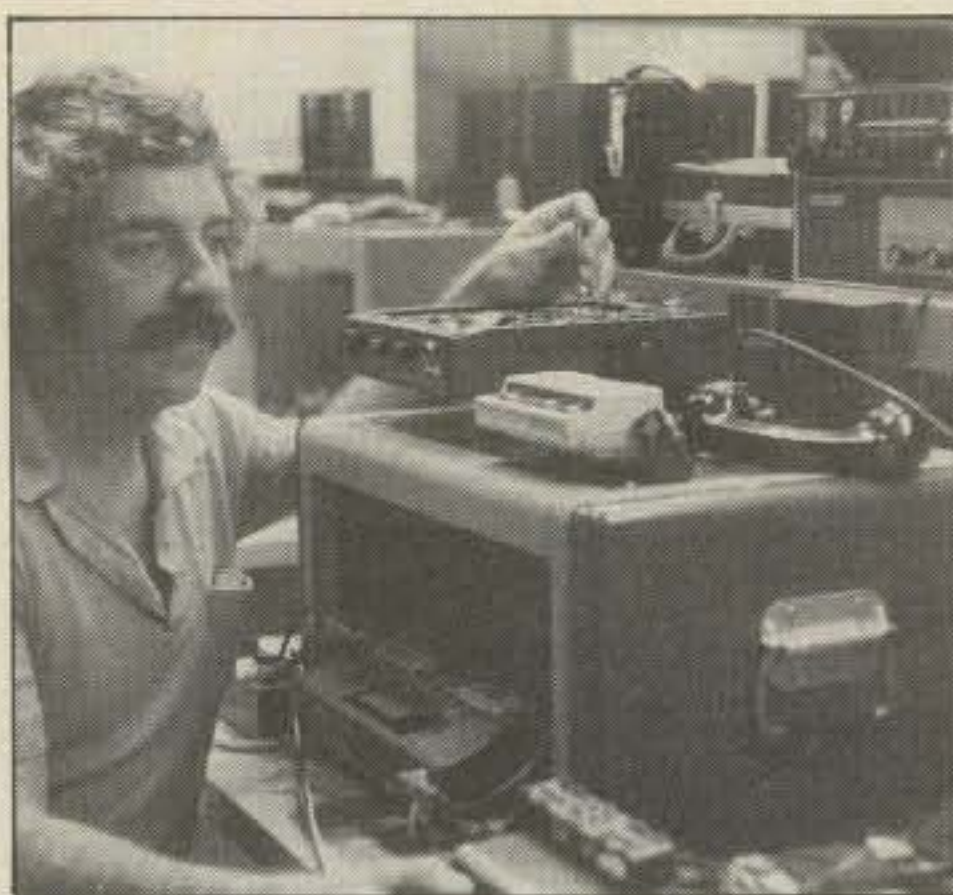
Engineer Hank Van Deursen adjusts ACSB equipment for testing of its effect on FM two-way radio.
