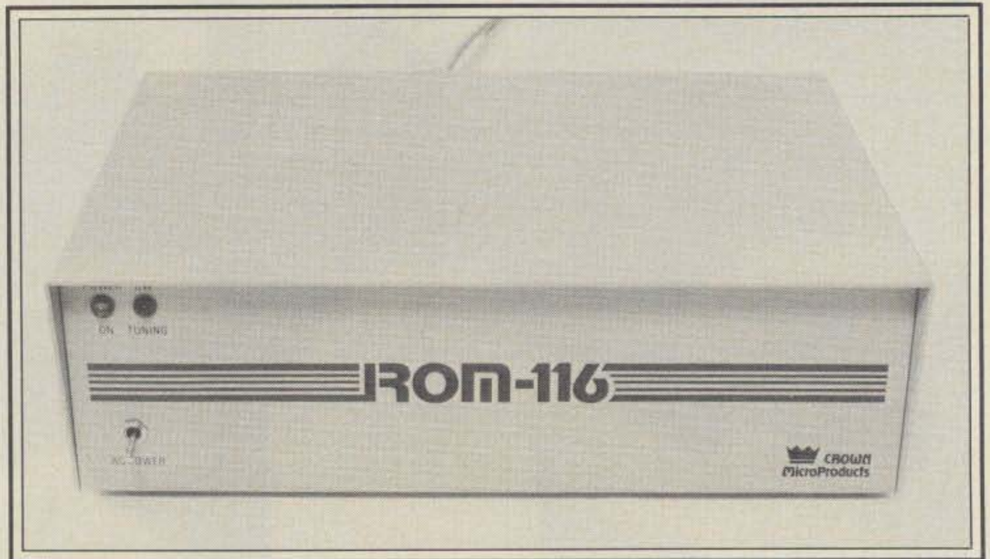
The ROM-116 front panel has the power switch at the left, and just above an LED for showing power on and another LED for indicating when c.w. signals are correctly tuned. The unit measures 3" x 7" x 10".
