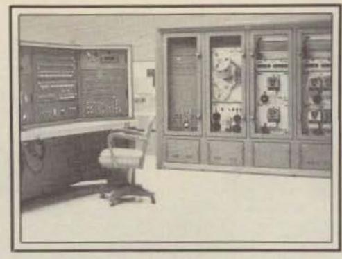
This early, 1956-model Burroughs guidance computer was the first operational unit to use transistors rather than tubes. The Burroughs computer was known as the Atlas Guidance Computer, Mod I.
