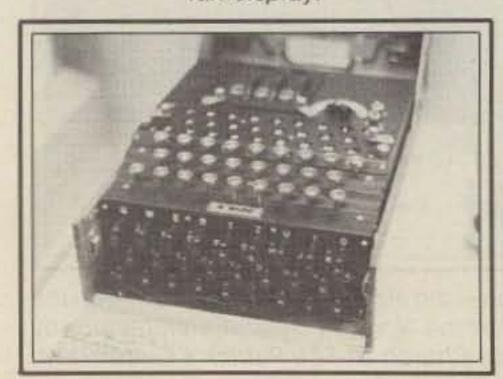
Amateur code breakers will be interested in this three-rotor German "Enigma" electromechanical cipher machine of World War II fame. The machine has no print capability, but it employs a 26-character light board to display, in turn, each ciphertext letter.
