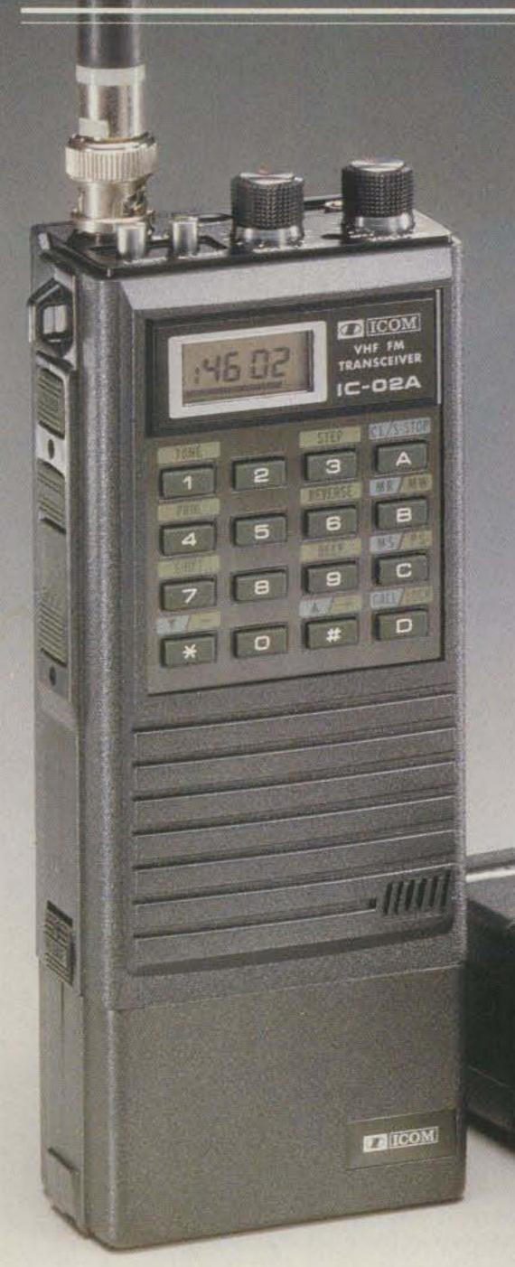
ICOM introduces the new top-ofthe-line IC-O2A and IC-O2AT to compliment its existing line of popular handheld transceivers and accessories. The new direct entry microprocessor controlled IC-O2A is a full-featured 2 meter handheld.
