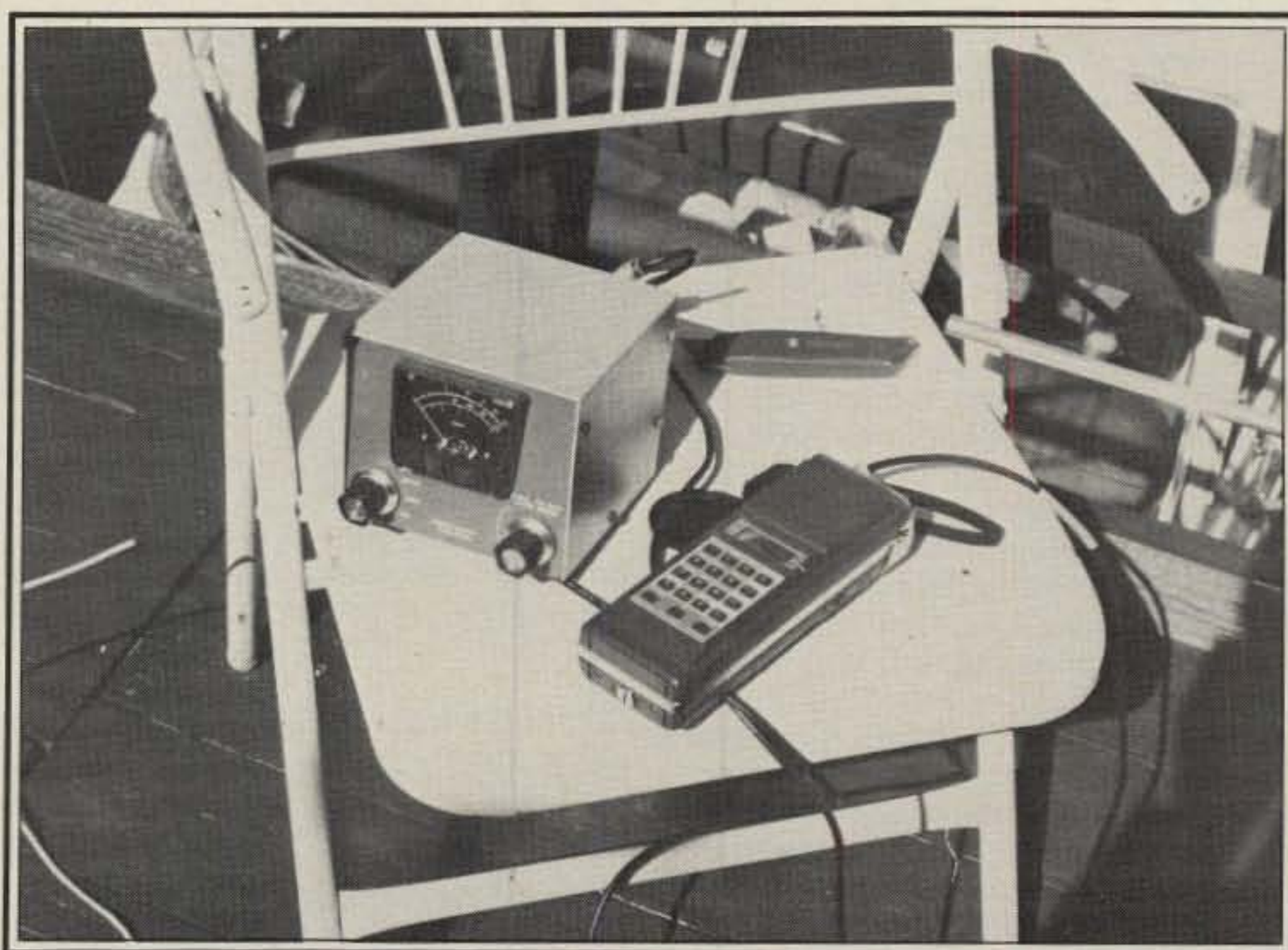
My test equipment is not very fancy, just a good s.w.r. bridge and transceiver.
