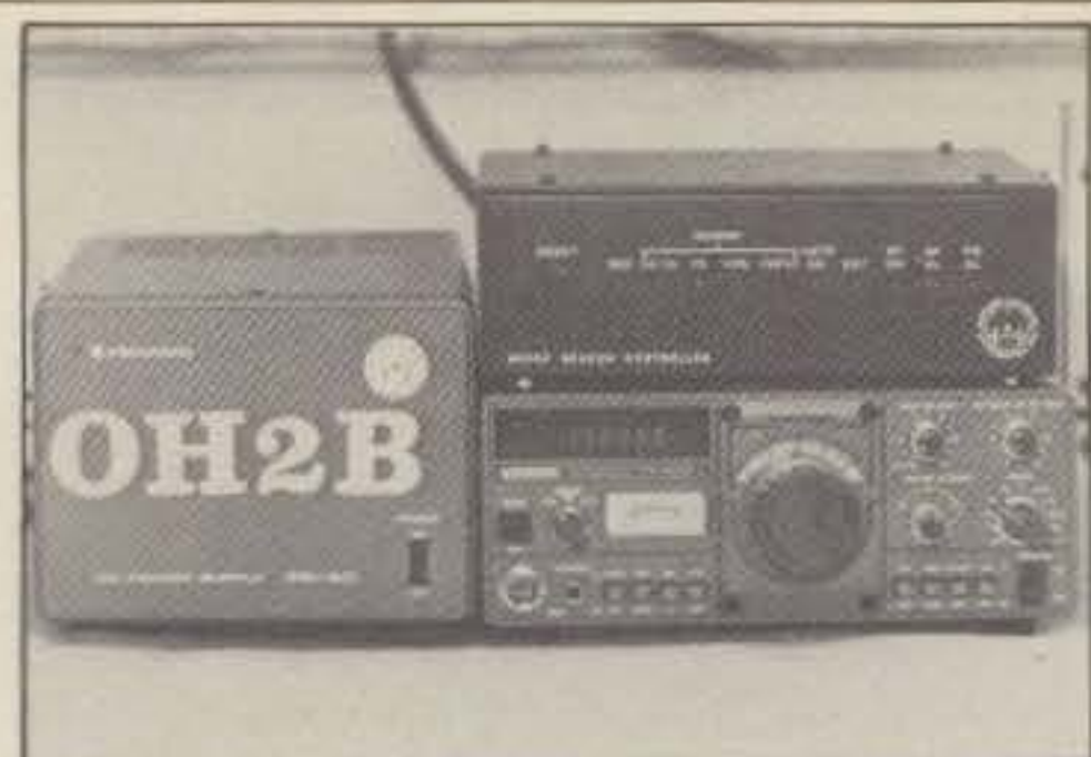
Close-up view of the OH2B system: a Kenwood TS130S, PS30 power supply, and the beacon controller.
