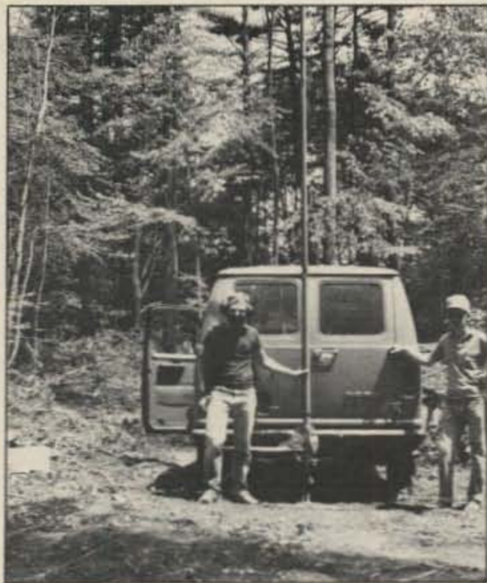
Tom, KR2V, and Carl, KA2GSM, on a logging road in NY. A 20 meter quad is mounted on the TV telescoping mast seen rising from the rear of the van. Tom didn't include details about the device on which the mast is mounted (center of bumper), but it looks like some bracket-winch designed especially for the job. Maybe he'll be kind enough to send in further details!
