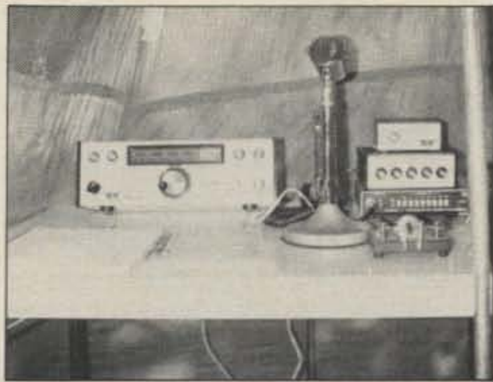
The classic-type QRP FD setup of Mike, KN7W. A portable table in a tent provides the operating position for the Argonaut with mike and keyer. Mike only turned seven s.s.b. QSOs, but is to be commended for bringing the mike along.
