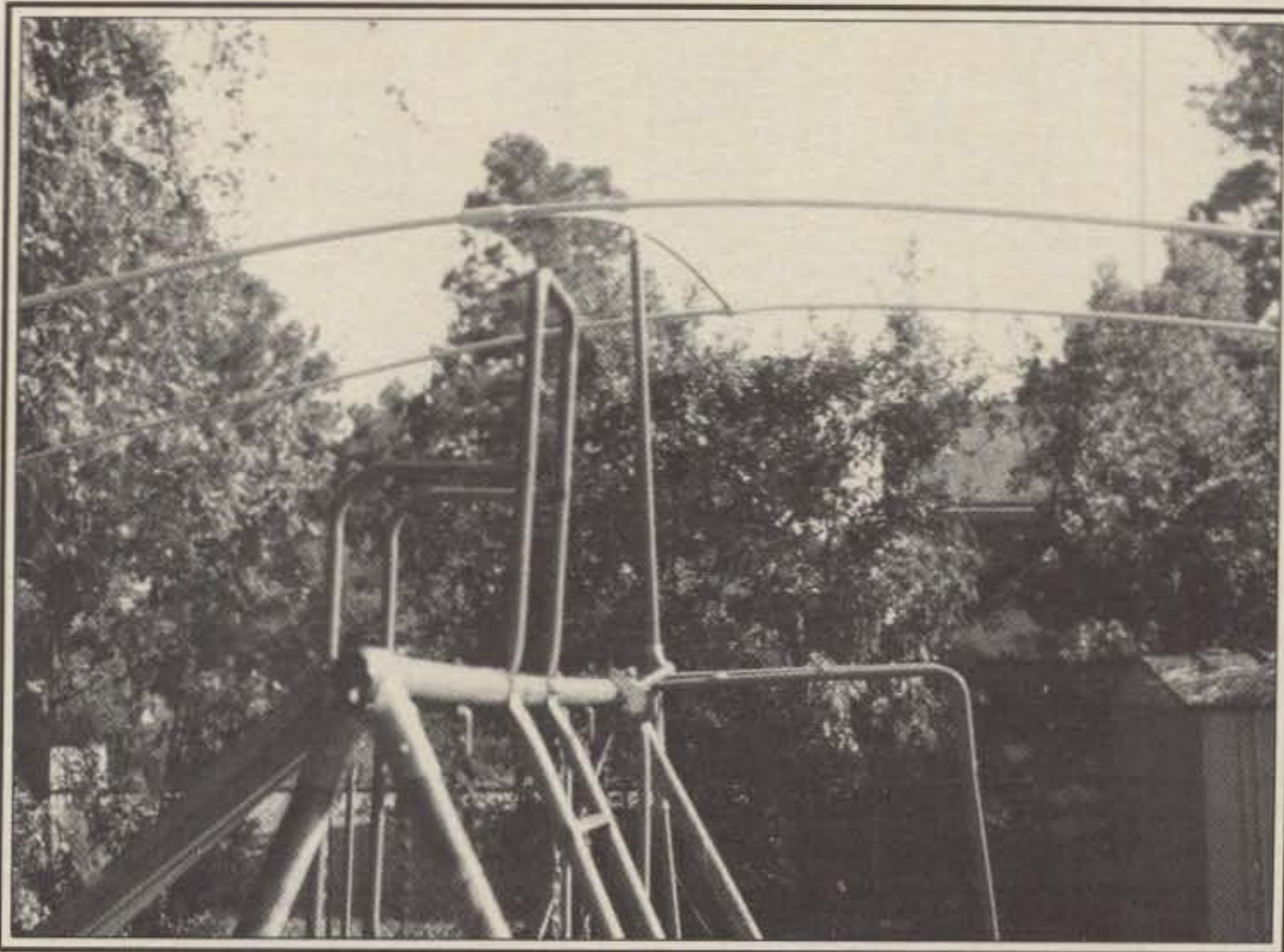
The completed beam antenna is installed on the N4HCR combination amateur radio tower/swing set for preliminary tests.
