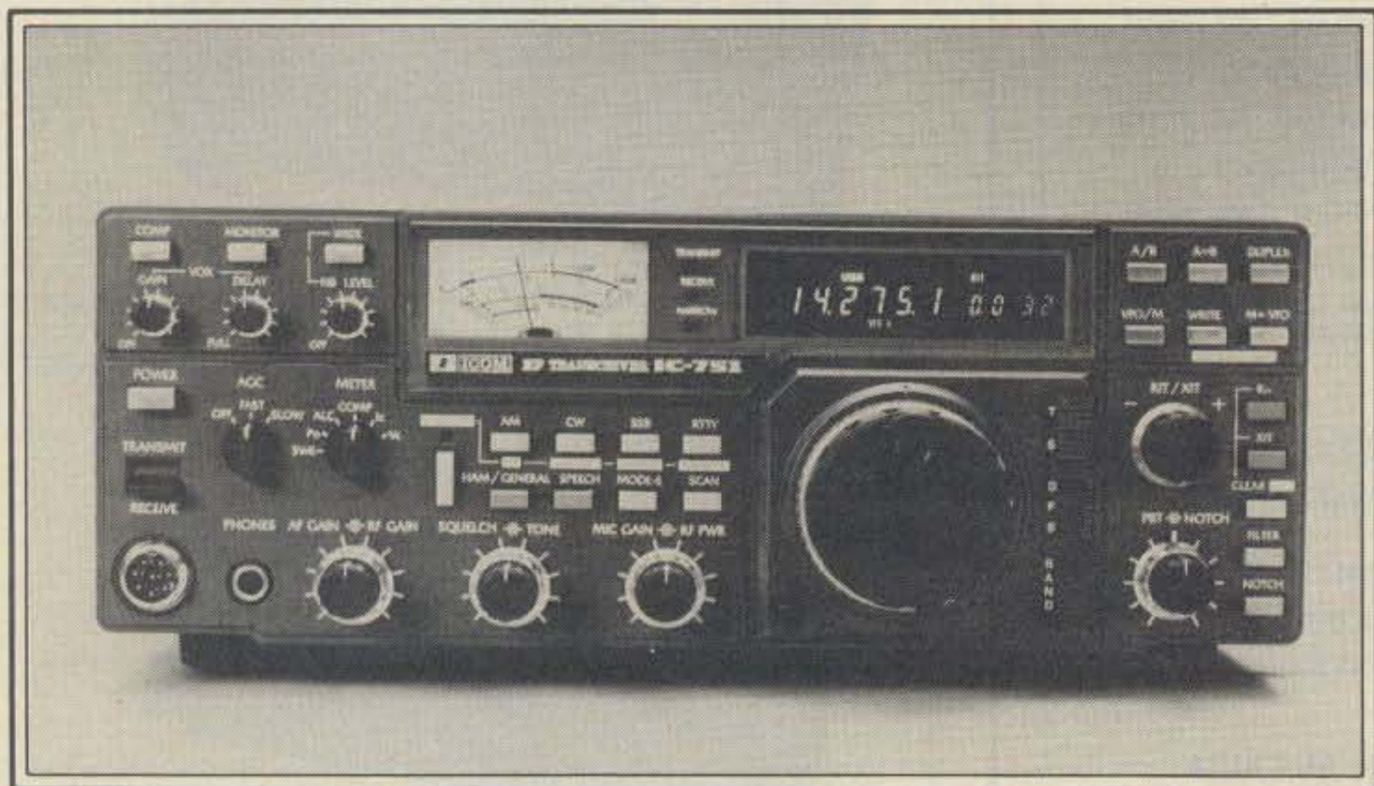
The front panel of the IC-751 is very well laid out. One hand can control all of the tuning/memory control functions.
