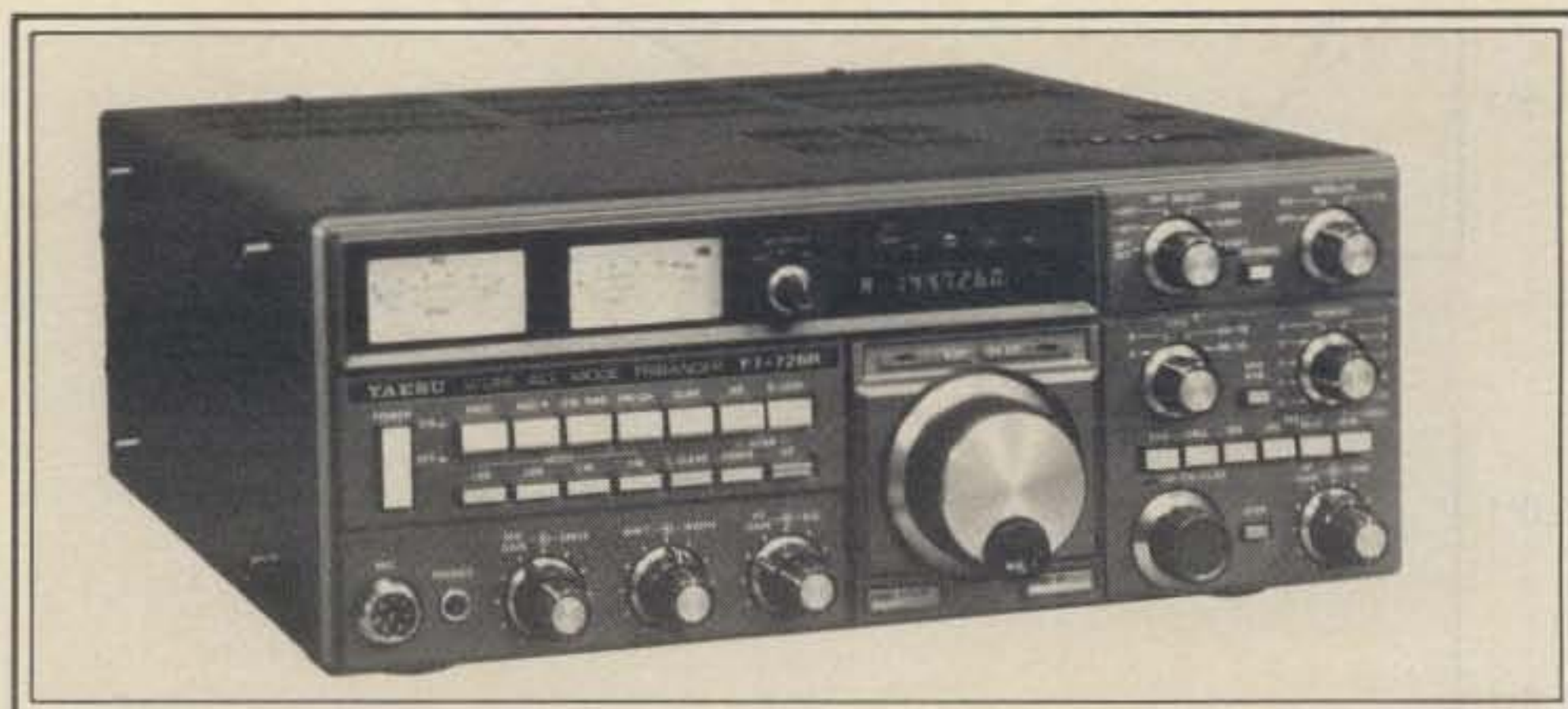
The Yaesu FT-726R 10 watt output, all-mode transceiver. As factory-supplied, the unit operates 2 meters only. Optional 70 cm and duplex modules are user-installed for satellite operation.
