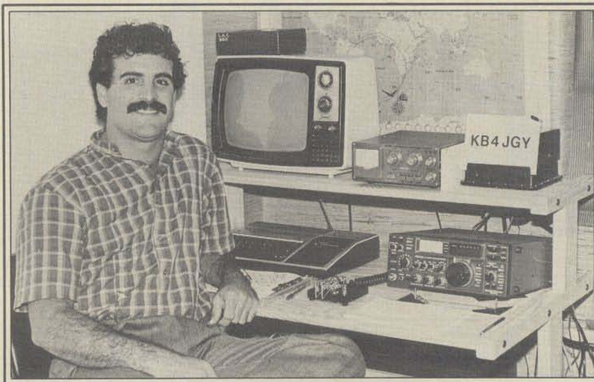
This is 24-year-old Louis A. Cruz, KB4JGY, a Miami police officer. He obtained his Novice license in March 1984, and he is getting ready to upgrade. His station includes an ICOM 745 transceiver, a Daiwa automatic antenna tuner, and a Bencher electronic keyer paddle. Louis operates on 10 or 15 meters most of the time, but he prefers 10 meters because it is less crowded.
