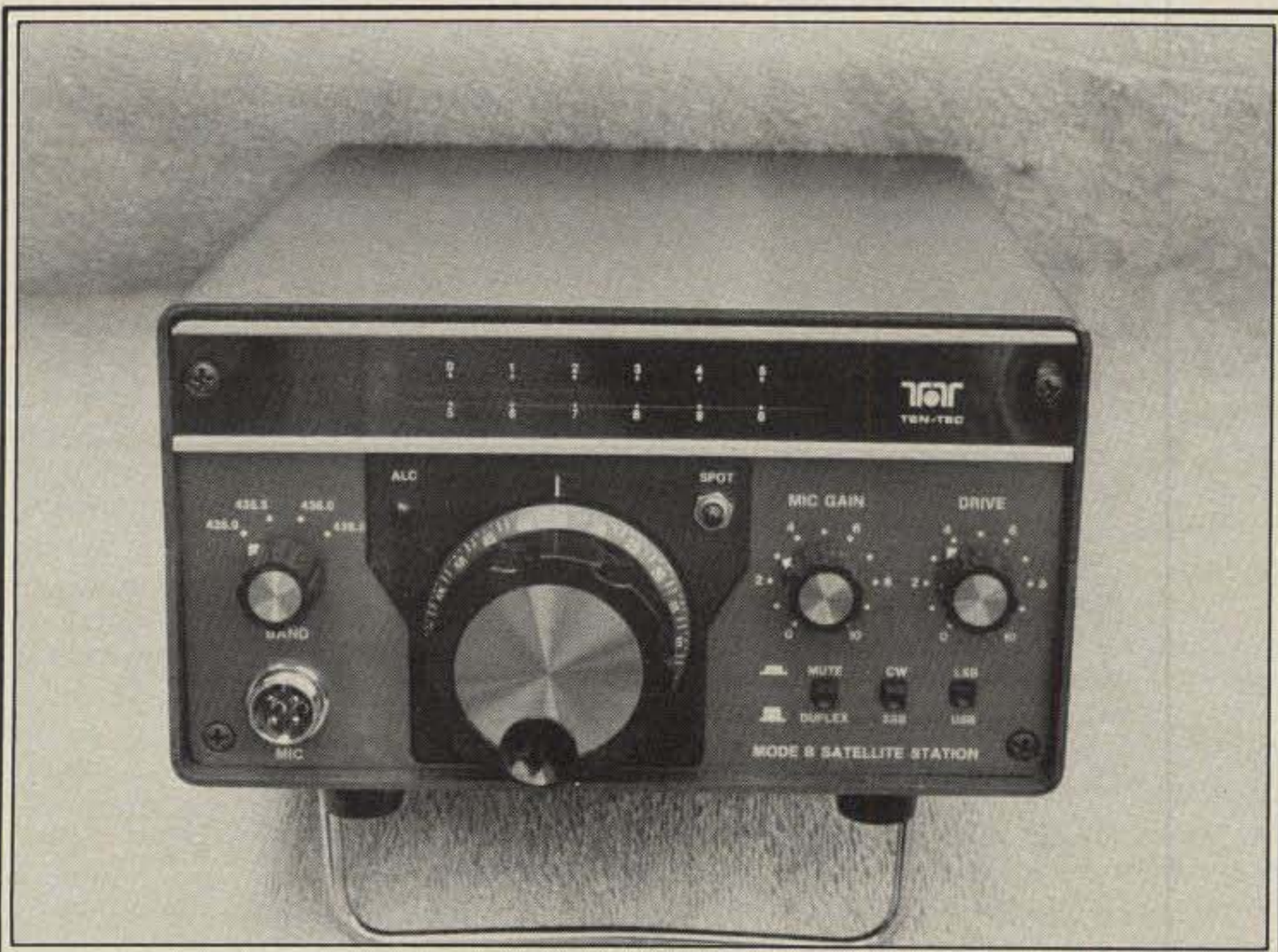
The Ten-Tec 2510 satellite station contains GaAsFET 2 to 10 meter converter and 70 cm c.w./s.s.b. transmitter in a single cabinet. The unit is used in conjunction with an h.f. transceiver or 10 meter receiver.
