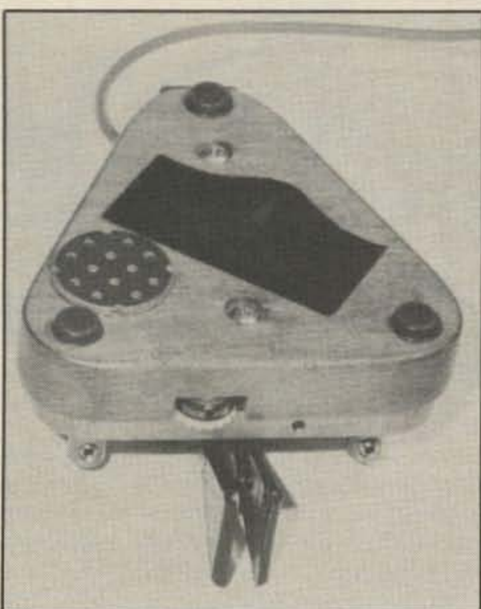
A bottom view of the completed keyer. A Vectorbord disc covers the hole for the crystal earphone, and the diagonal dark patch is the relocated, but apparently unphotogenic, Vibroplex label.
