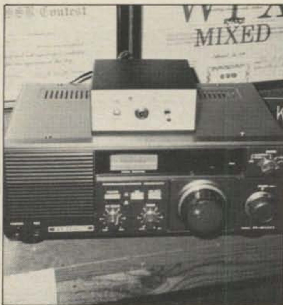
Photo of receive-only demodulator for c.w., RTTY, and ASCII atop the author's R600 general-coverage receiver.
