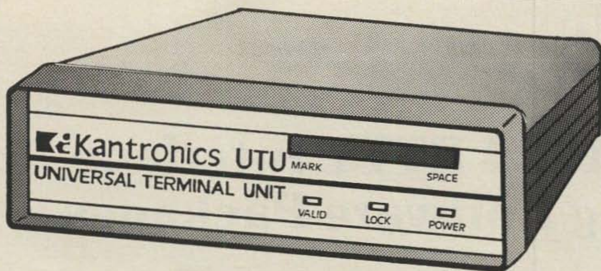
Fig. 3— A simple RTTY TU using a series of LEDs to indicate mark and space.
