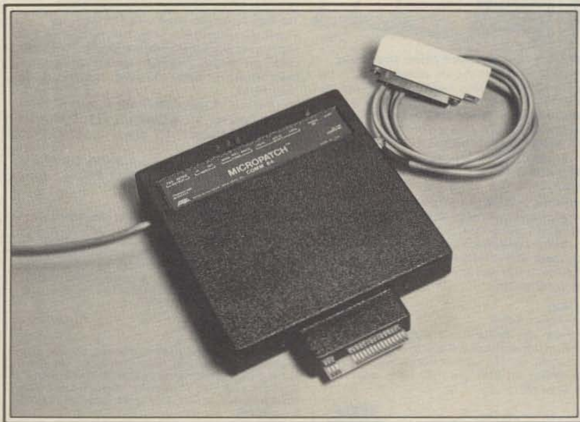
A recent approach to printed-word interfacing between transceivers and home computers consists of plug-in multi-mode adapters such as AEA's Micropatch. This compact unit fits directly into the Commodore 64 and provides RTTY, c.w., and AMTOR operations. Language conversions and data checking are under software control.
