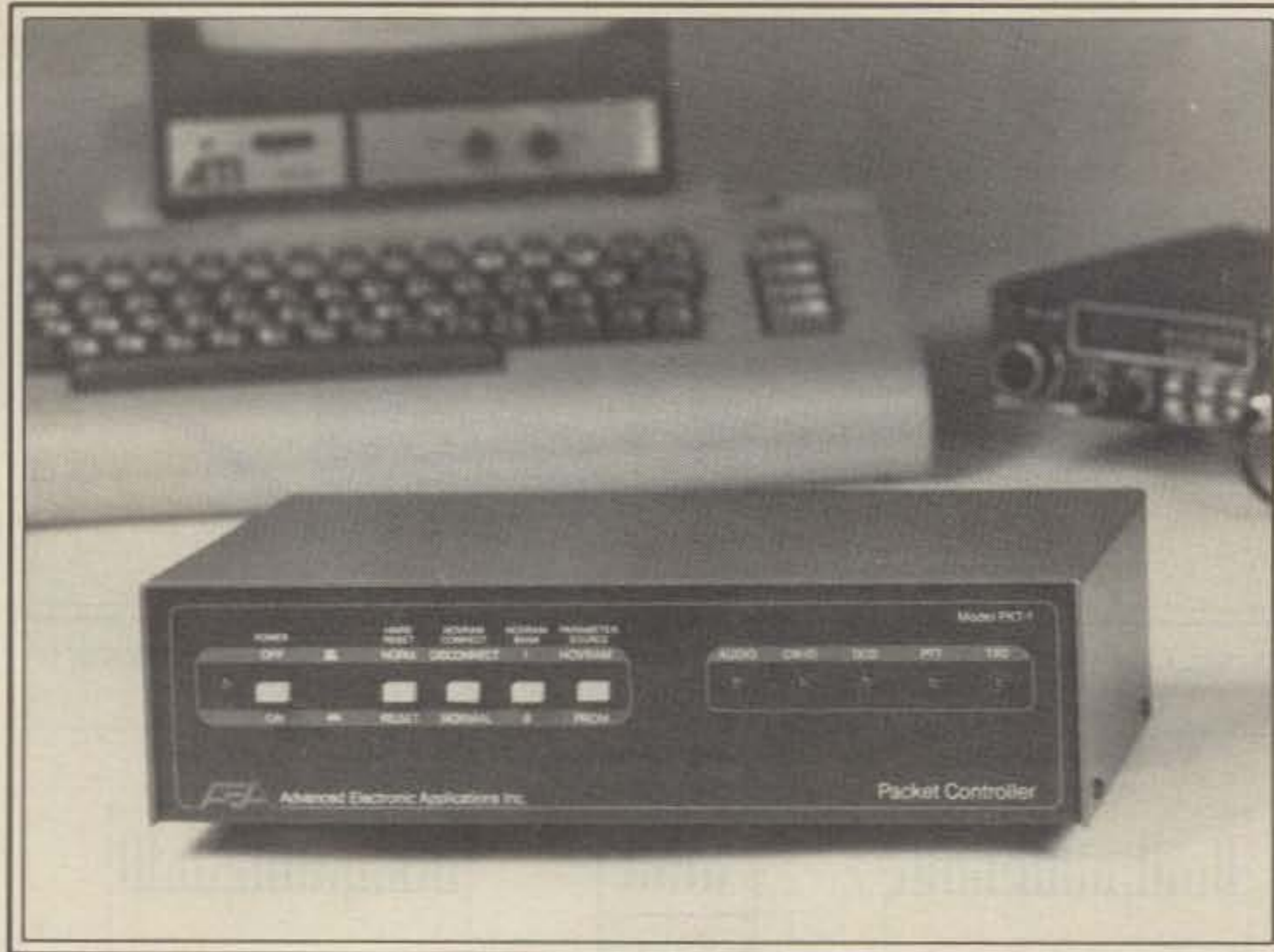
Items used for joining the activity of an amateur radio packet network. Setup consists of AEA (or equivalent) packet controller, home computer with terminal program, and v.h.f. transceiver. Multiple QSOs are conducted on a single frequency using time multiplexing techniques.
