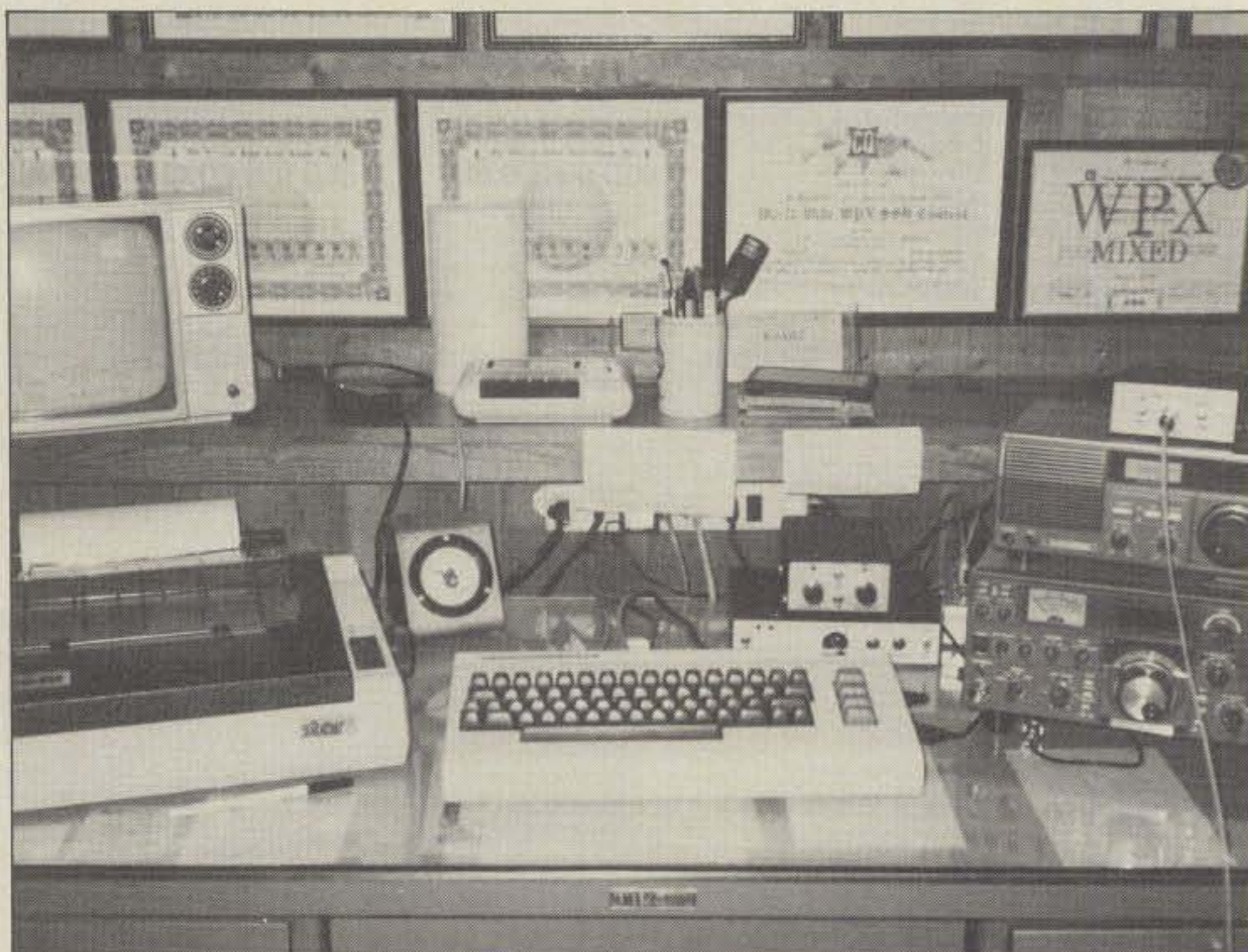
The author's complete RTTY station, including VIC-20, monitor, Gemini 10X printer, c.w.-RTTY active filter, home-brew modem, receive-only demodulator, TS-530S transceiver, and R600 receiver.
