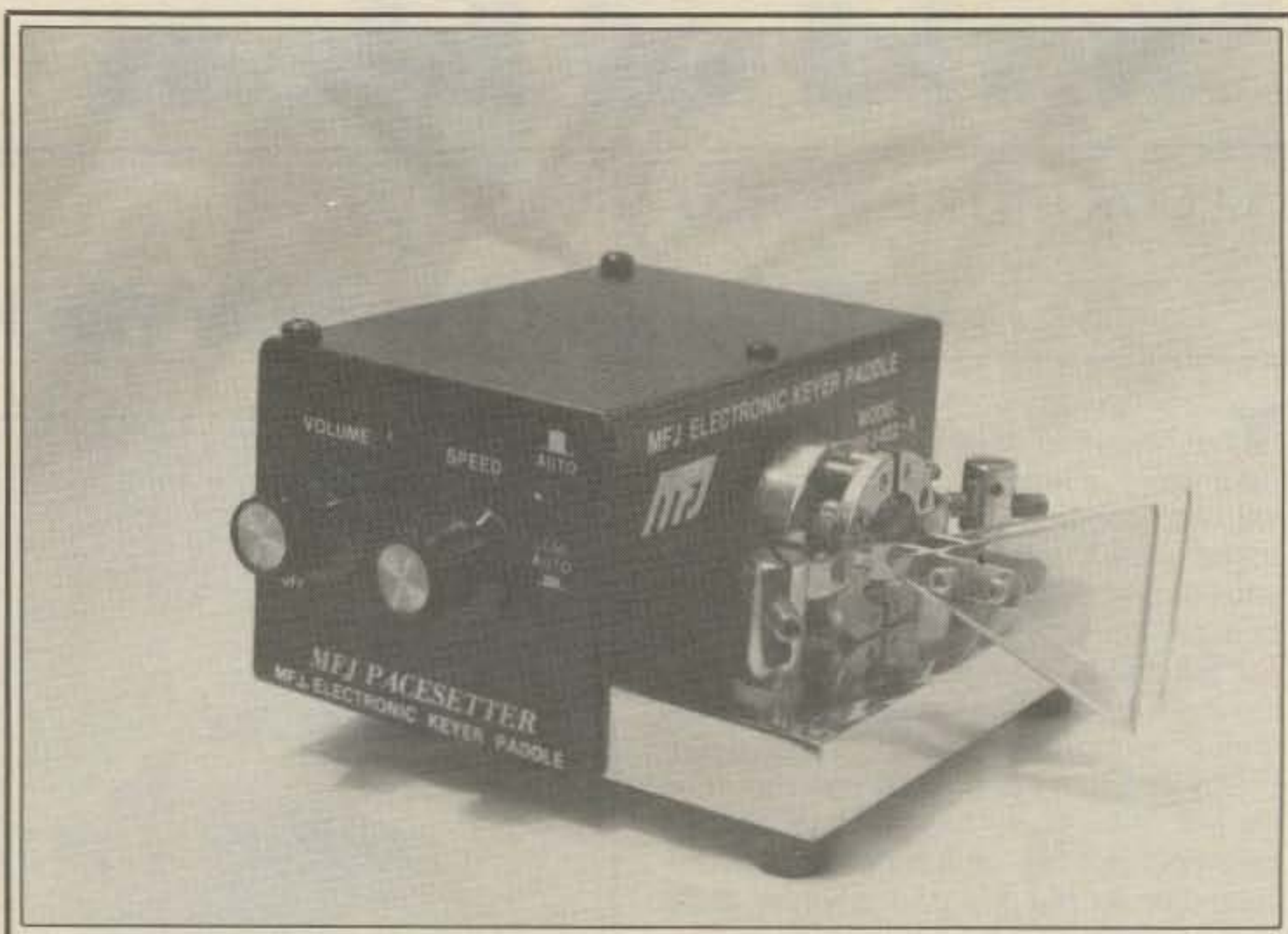
If your c.w. is a mite rusty, renew interest with a smooth operating electronic keyer and paddle. This MFJ/Bencher combo is fully portable and features iambic operation with dot/dash memory.
