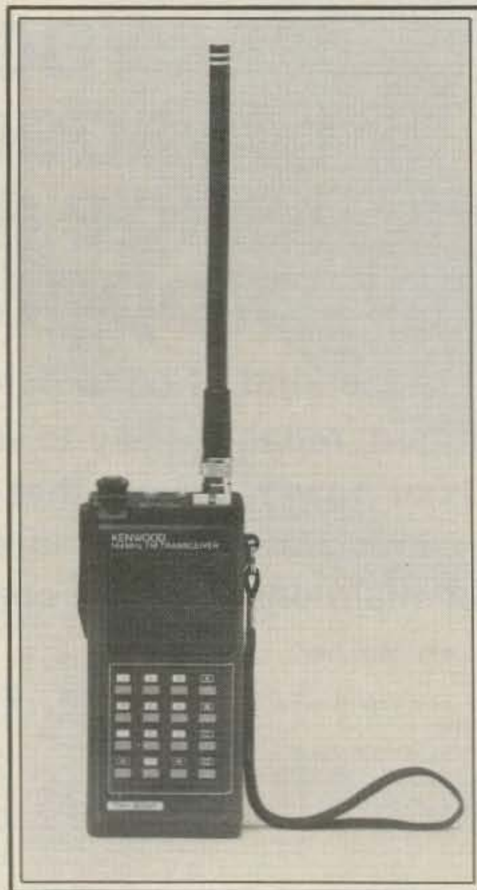
The Kenwood TH-21AT Tiny Talkie. Unit is approximately the size of a pack of cigarettes, tunes 144.00 to 148.95 MHz, and runs 1 watt output.
