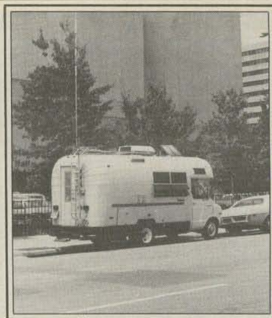
The principles of vertical-antenna installations for use on mobile homes and recreational vehicles are the same as for fixed installations. In both cases it's important to erect the vertical in the clearest possible spot, and to install the best possible ground system beneath the antenna. (W8FX photo)
