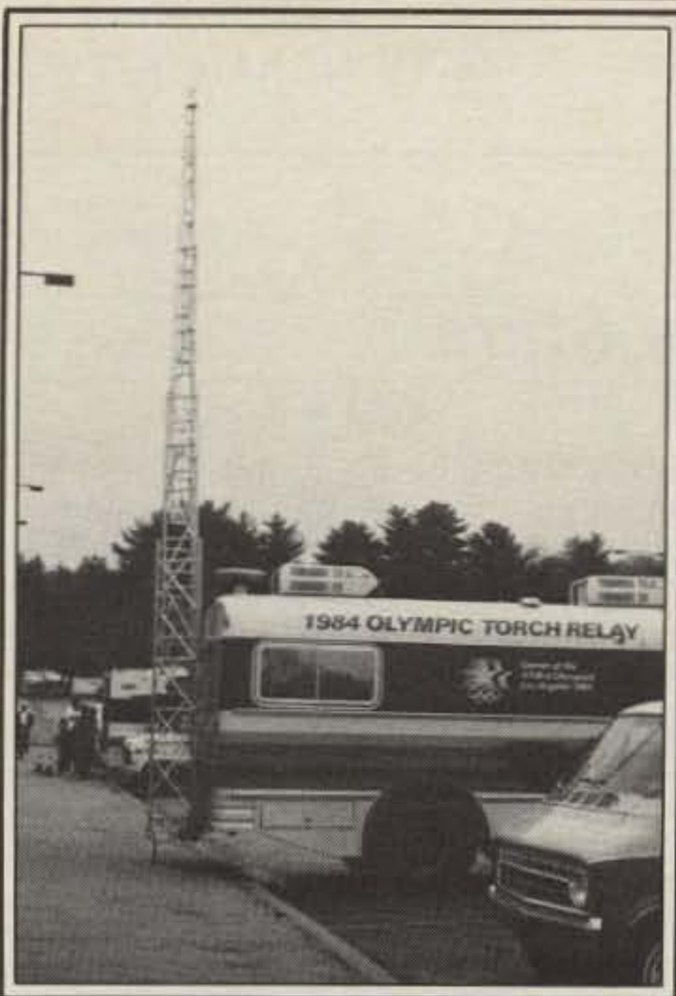
This Olympic Torch Relay communications vehicle used in the 1984 Olympics torch-carrying route sports an Aluma Towers Model BD-150, 50 ft. crank-up tower partially extended (the vehicle belongs to AT&T). The vehicle was used as a communications center for the 30 or so vehicles involved in the torch-carrying run. In a matter of a few minutes the tower can go from the traveling position to being fully extended and on the air.
