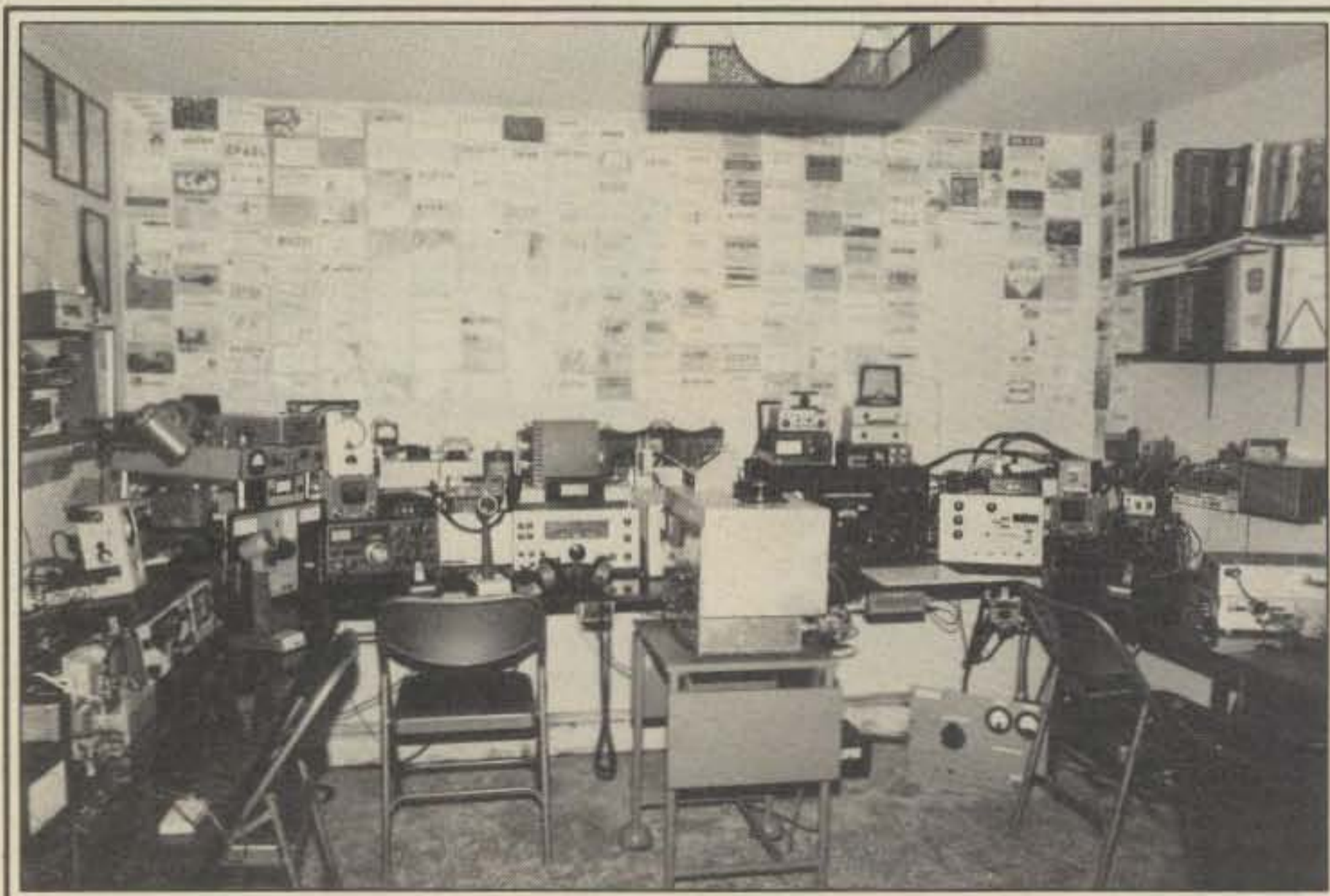
Some of the VHF/UHF station at WB2WIK. The 30 foot long operating bench covers three walls in "wraparound" fashion and supports gear for from 50-1296 MHz.
