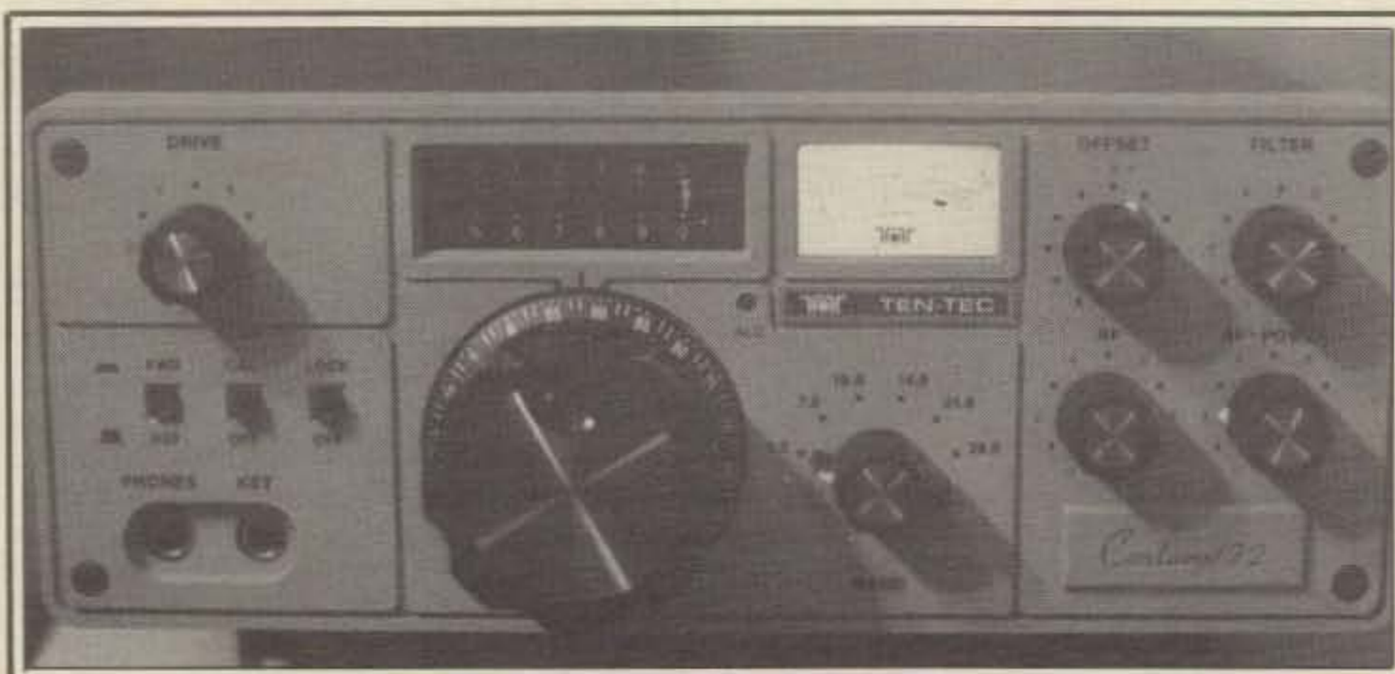
The Ten-Tec Century 22 six-band CW-only transceiver. The unit sports full break-in and double-direct conversion receiver.
