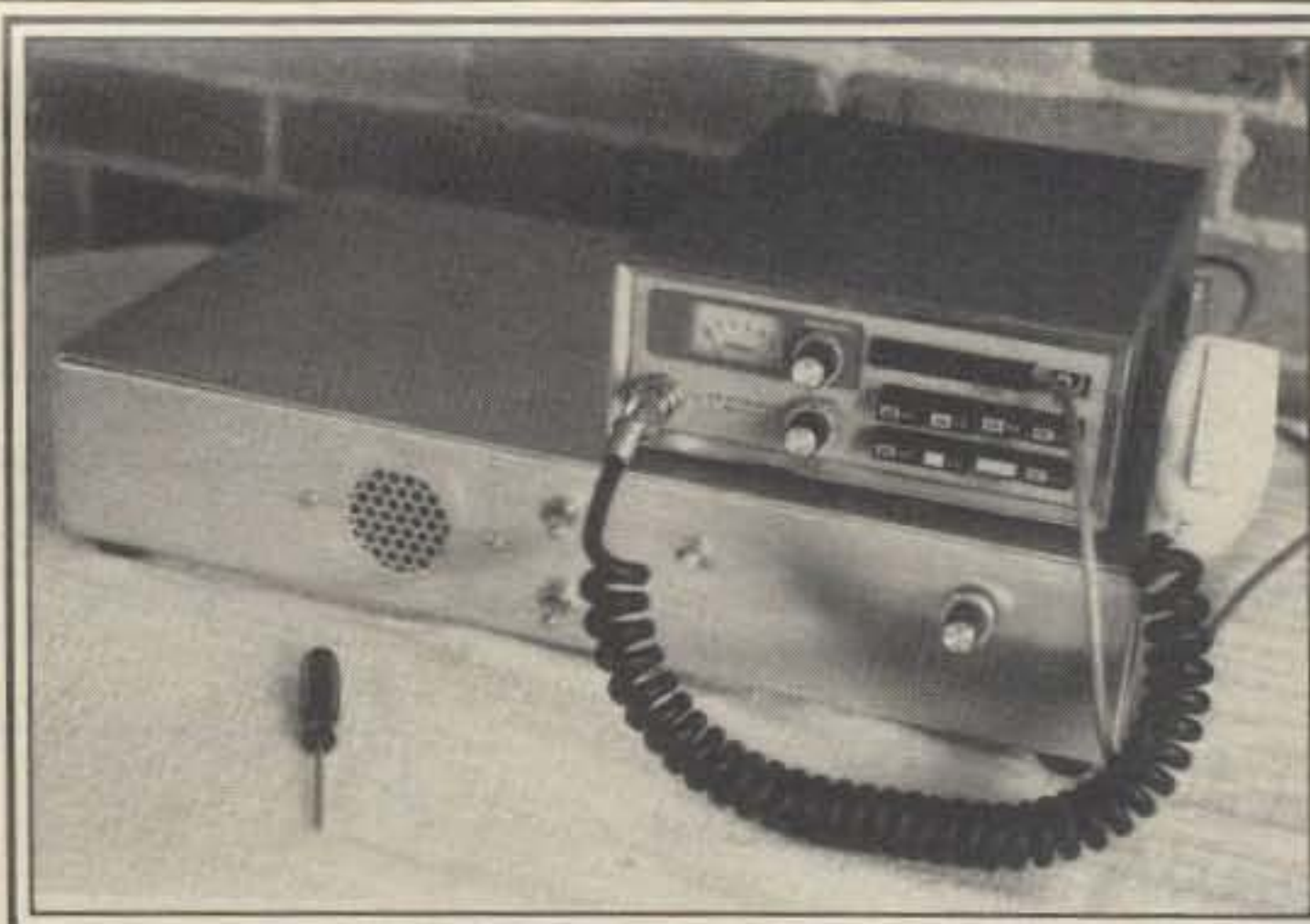
Complete 2 meter repeater. Local speaker and microphone add to on-site adjustments.
