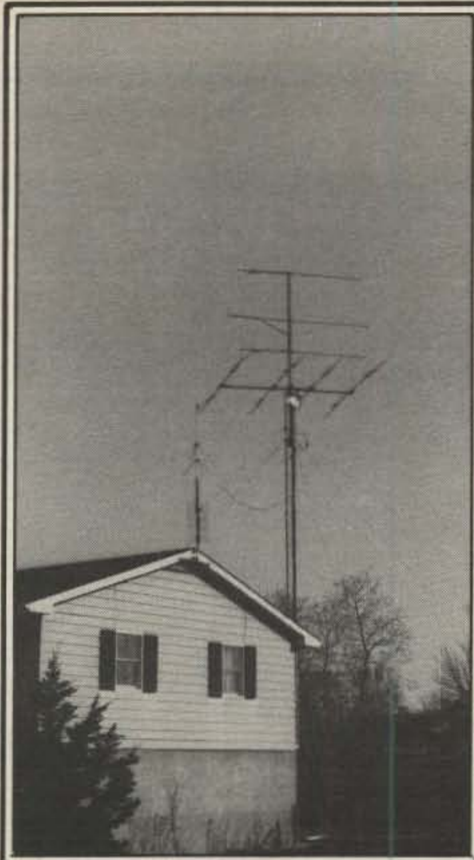
Antenna farm at WB9MSV: 14/14-element "Jr. Boomers" on 144 MHz, with a 24-element "Boomer" for 70 cm stacked between the 2 meter Yagis. Below is a 4-element KLM tribander.
