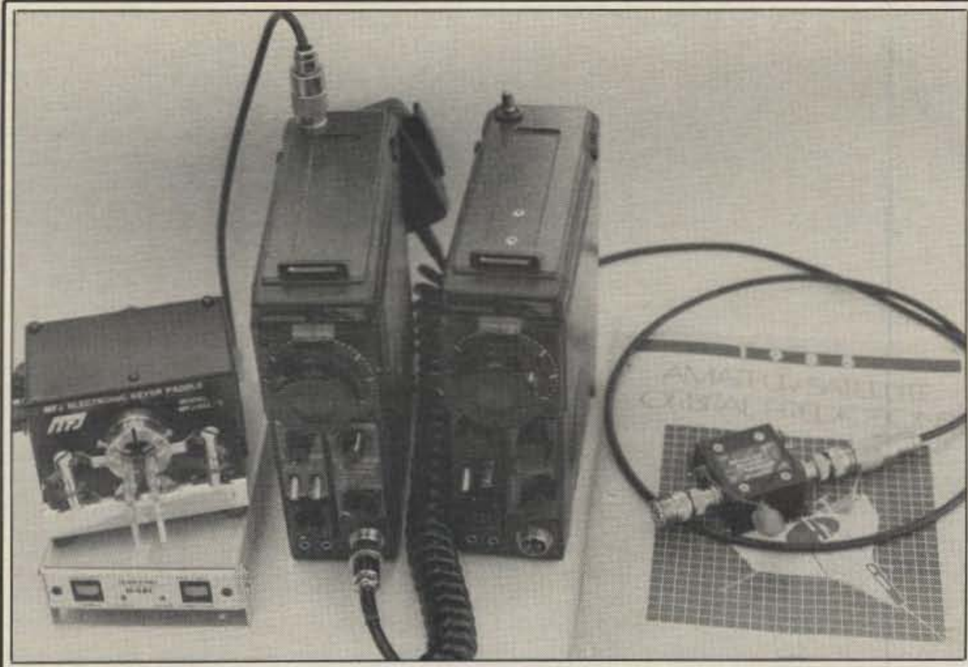
Fig. 2— Essential items of a "bare bones" OSCAR 10 setup for mode B operation. ICOM 202 portable 2 meter SSB/CW transceiver is mated with GaAsFET preamp, while ICOM 402 portable 70 cm SSB/CW transceiver drives Encomm/Tokyo HL32U 20 watt amplifier. Add "twist" antennas for each band and the setup is capable of worldwide communications. (Setup is K4TWJ's backup/portable rig.)
