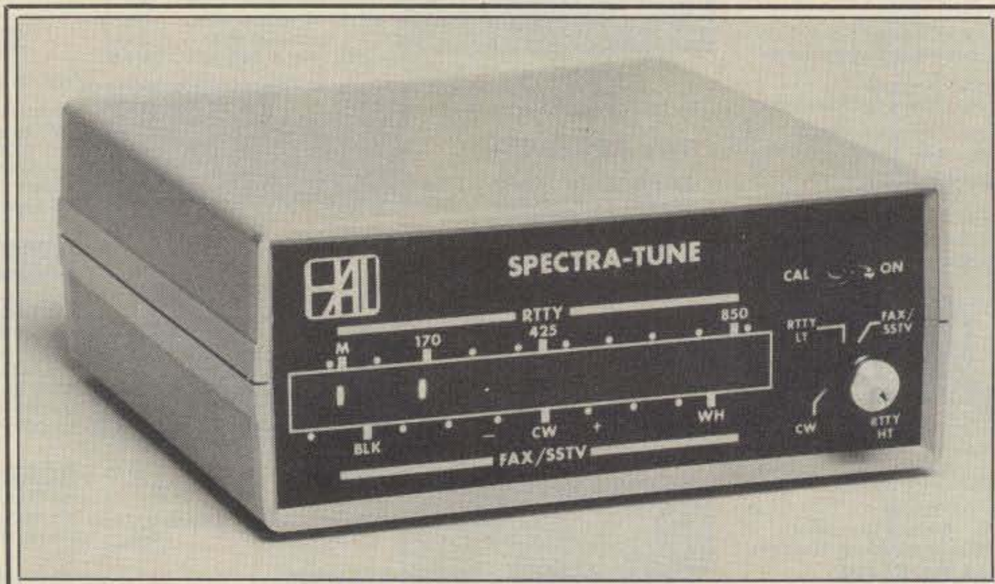
The HAL Communications Spectra-Tune, a compact and effective tuning indicator for RTTY, ASCII, and SSTV.
