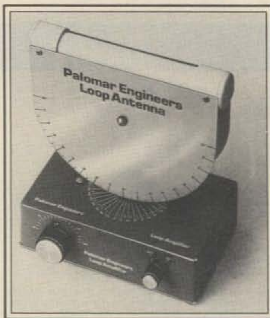
Small directional loops make excellent receiving antennas, particularly when used in tandem with a low-noise preamplifier. Indoor antennas of this type are very popular with 160 meter ops, broadcast band DXers, and VLF ("lower") enthusiasts because of the extreme directivity of the antennas and the ability to null out interference and noise. (Photo courtesy Palomar Engineers)
