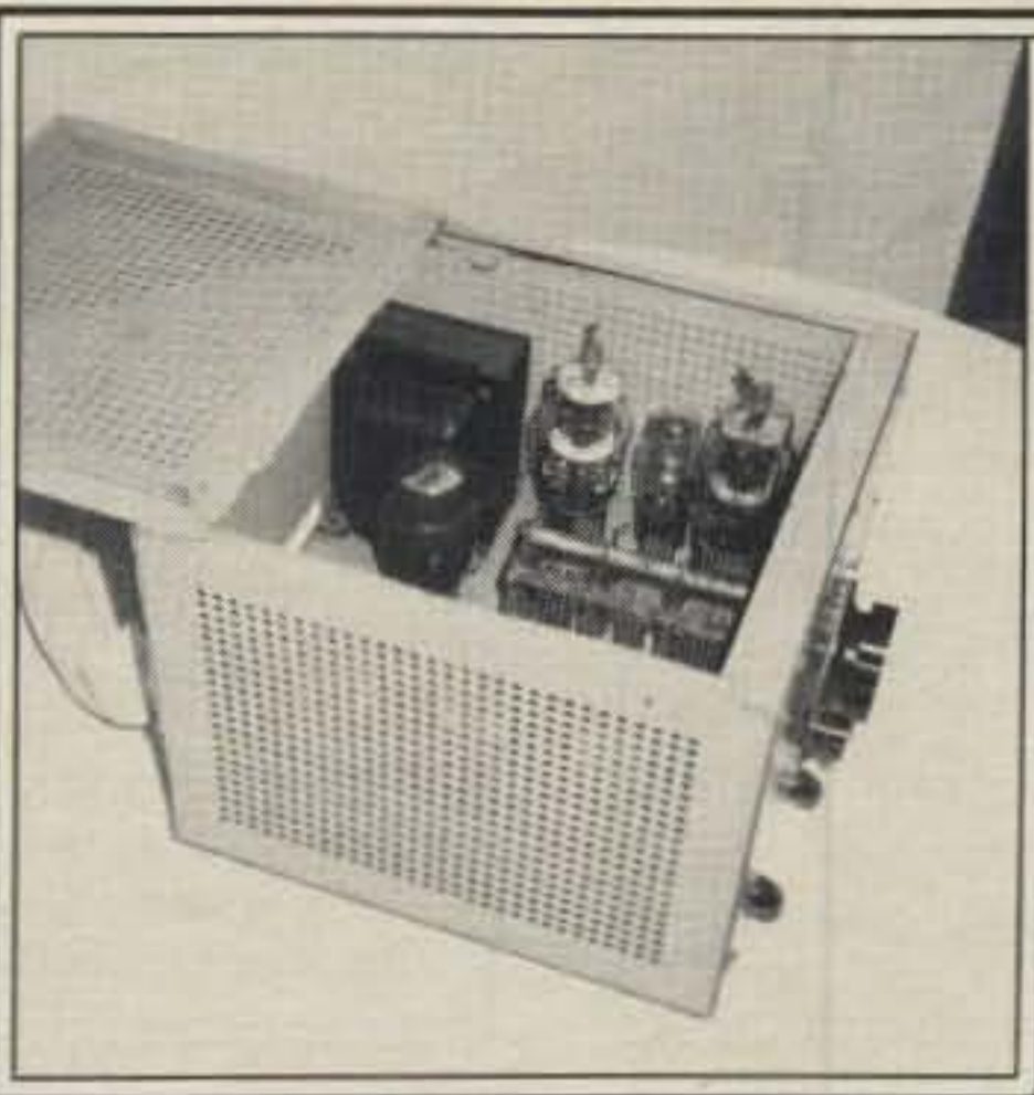
This transmitter, using push-pull 807s and a 6L6 VFO, is similar to the one Willard carried around the world. (Tnx W6PN)
