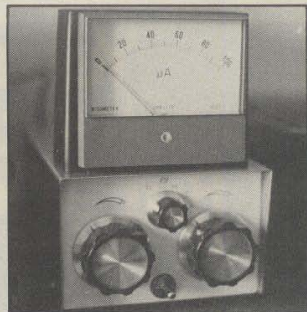
SWR meter follies. One advantage of having the reflectometer circuitry inside the tuner but the meter external is that one can experiment with different style meters. Here, a rather giant size meter is being used almost half as large as the tuner itself.
