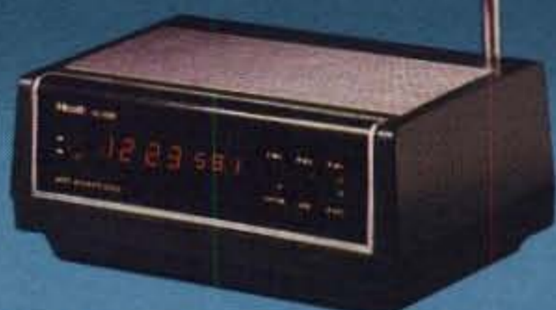
Most Accurate Clock uses NBS atomic clock signal to keep "perfect" UTS time.
