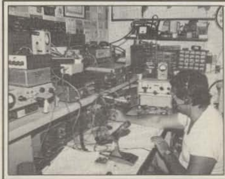
This is KC2PX operating the 432 MHz station at NV6O/2. We used a TS830S + MMT432/28S transverter driving a Mirage intermediate amplifier, to drive a Henry 2004 kw amp (3CX800A7, 650 watts out). The RX used a mast-mounted SSB Electronics GaAsFET preamp. Also visible here are stations for 220 and 1296 MHz.
