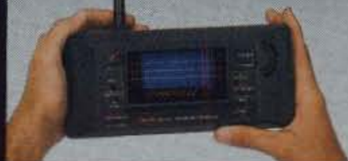
World's first low-cost hand-held, microprocessor-controlled Real Time Spectrum Analyzer.
