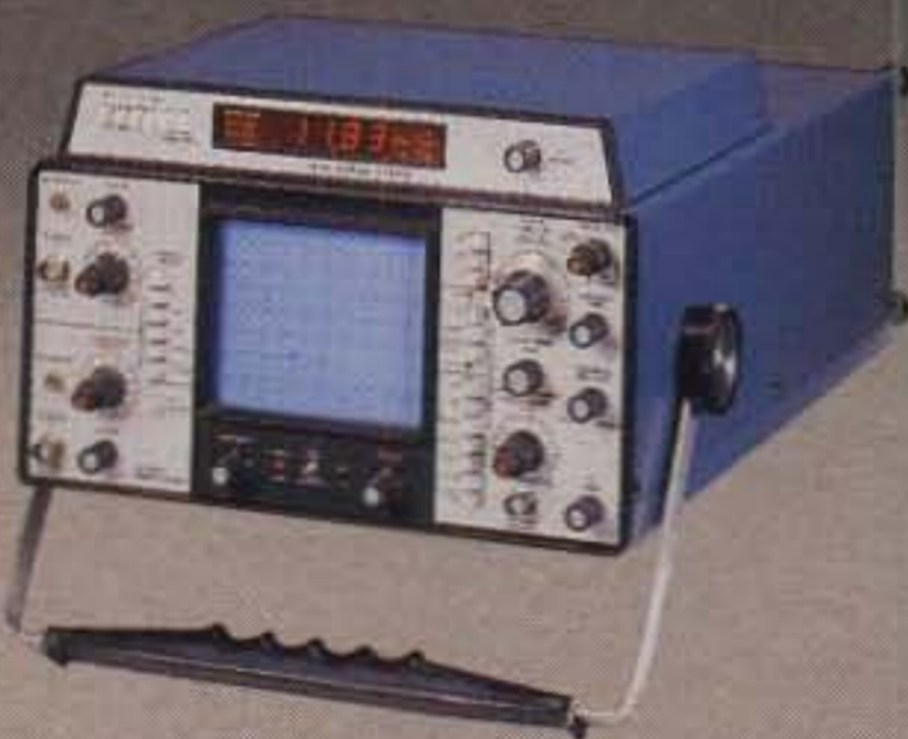
Triple-trace oscilloscope speeds troubleshooting.
