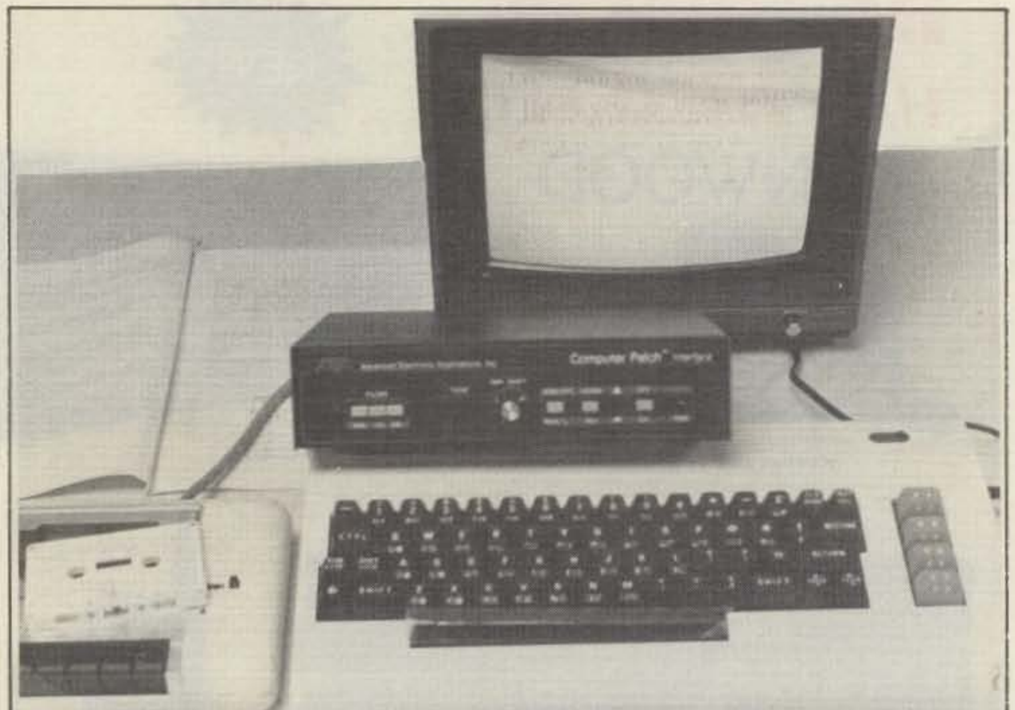
Fig. 2—Equipment used in assembling the basic computerized RTTY/CW/ASCII system shown in fig. 1. Cassette software included in this example.
