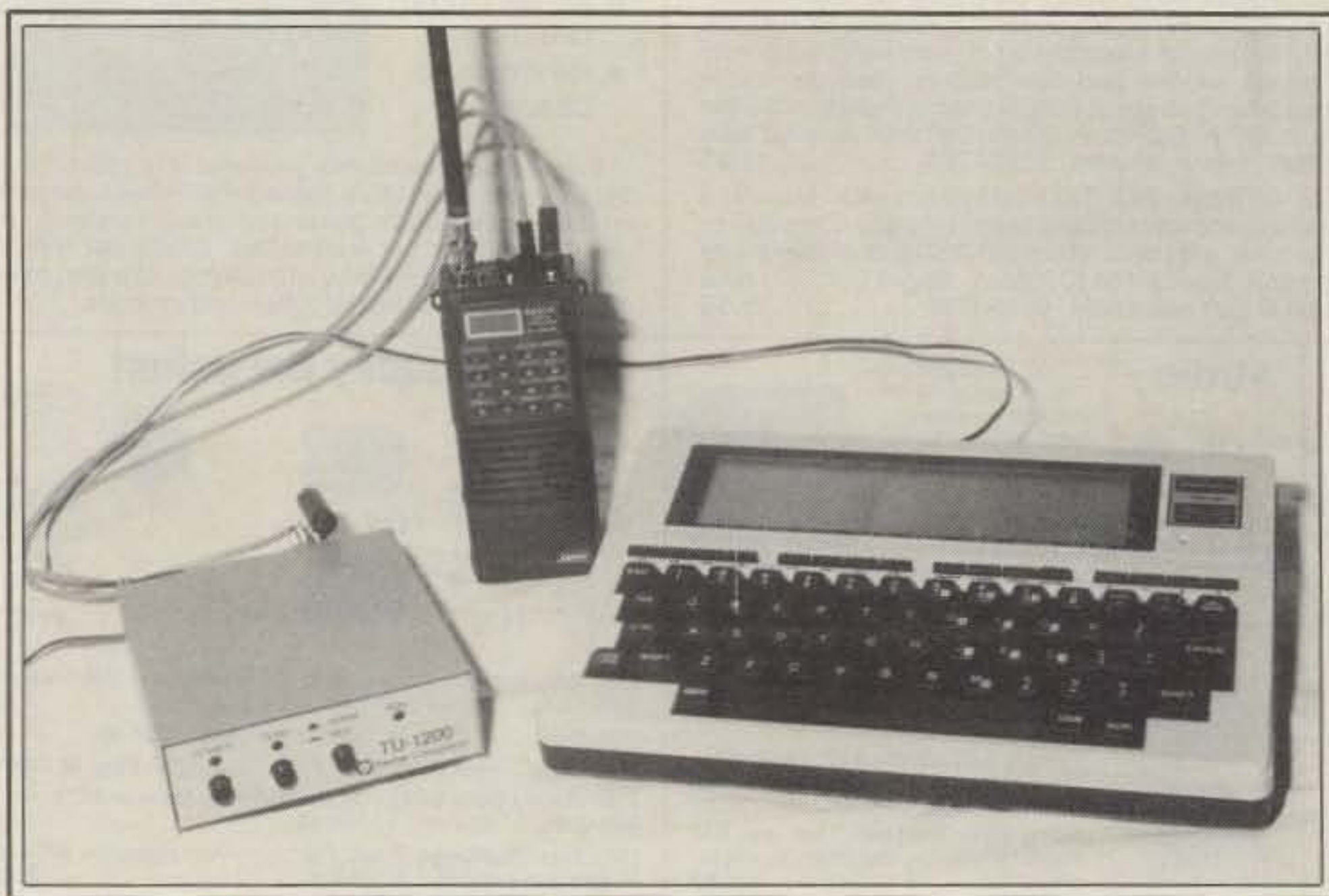
A simple, portable RTTY station consisting of a Flesher TU-1200, an ICOM 02-AT, and a Radio Shack® TRS-80 Model 100.
