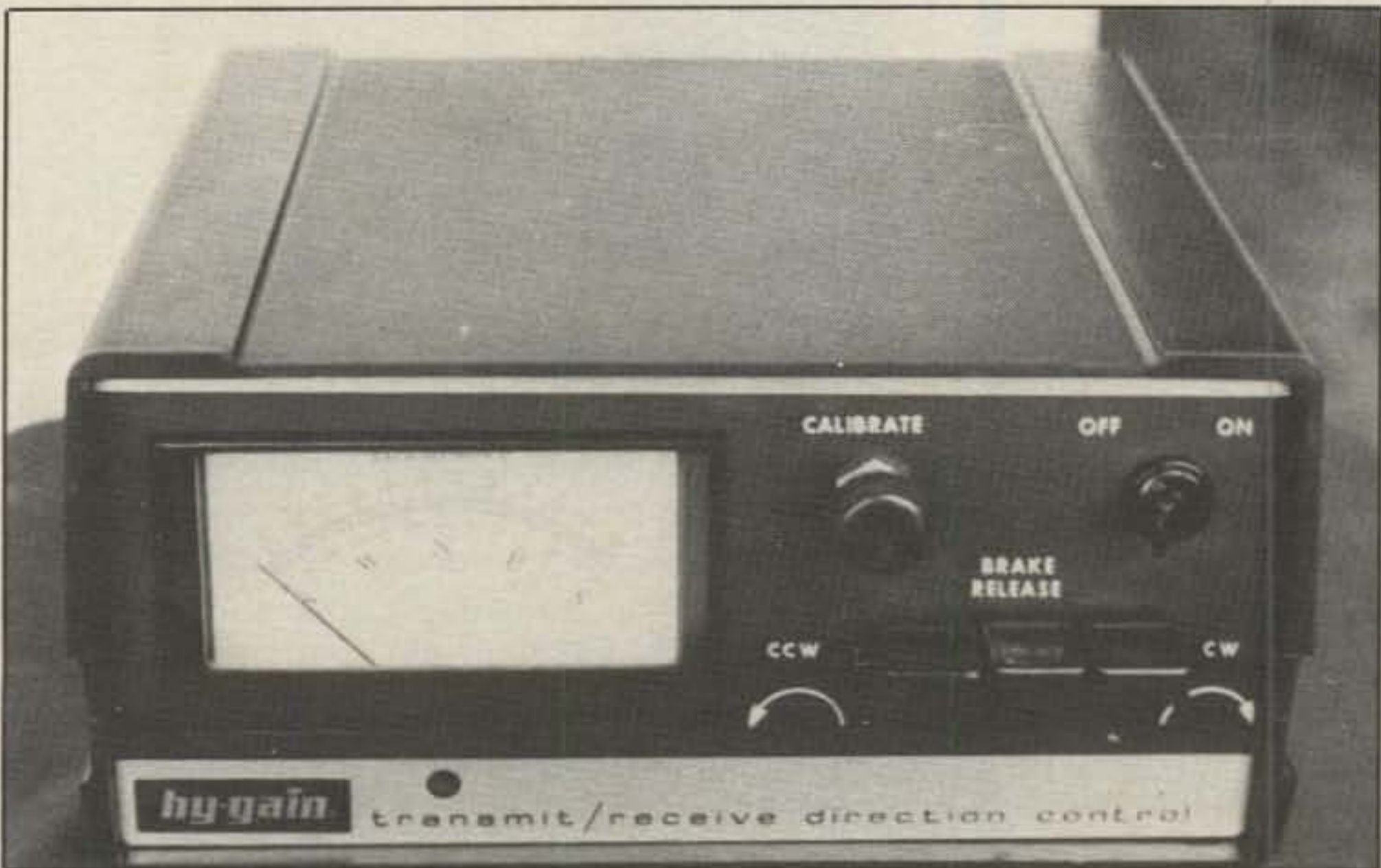
The control unit is housed in a smartly styled plastic/metal enclosure. The meter center is north, but the scale can be reversed to show south as center.
