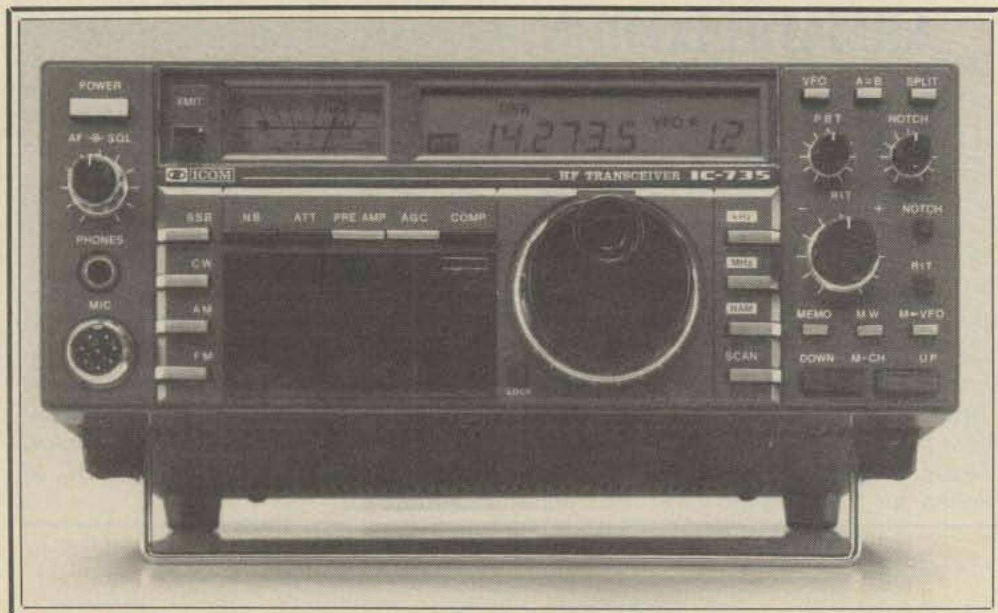
The ICOM 735 HF transceiver with general-coverage receiver and numerous special features. Unit is quite compact and a true dream to operate.
