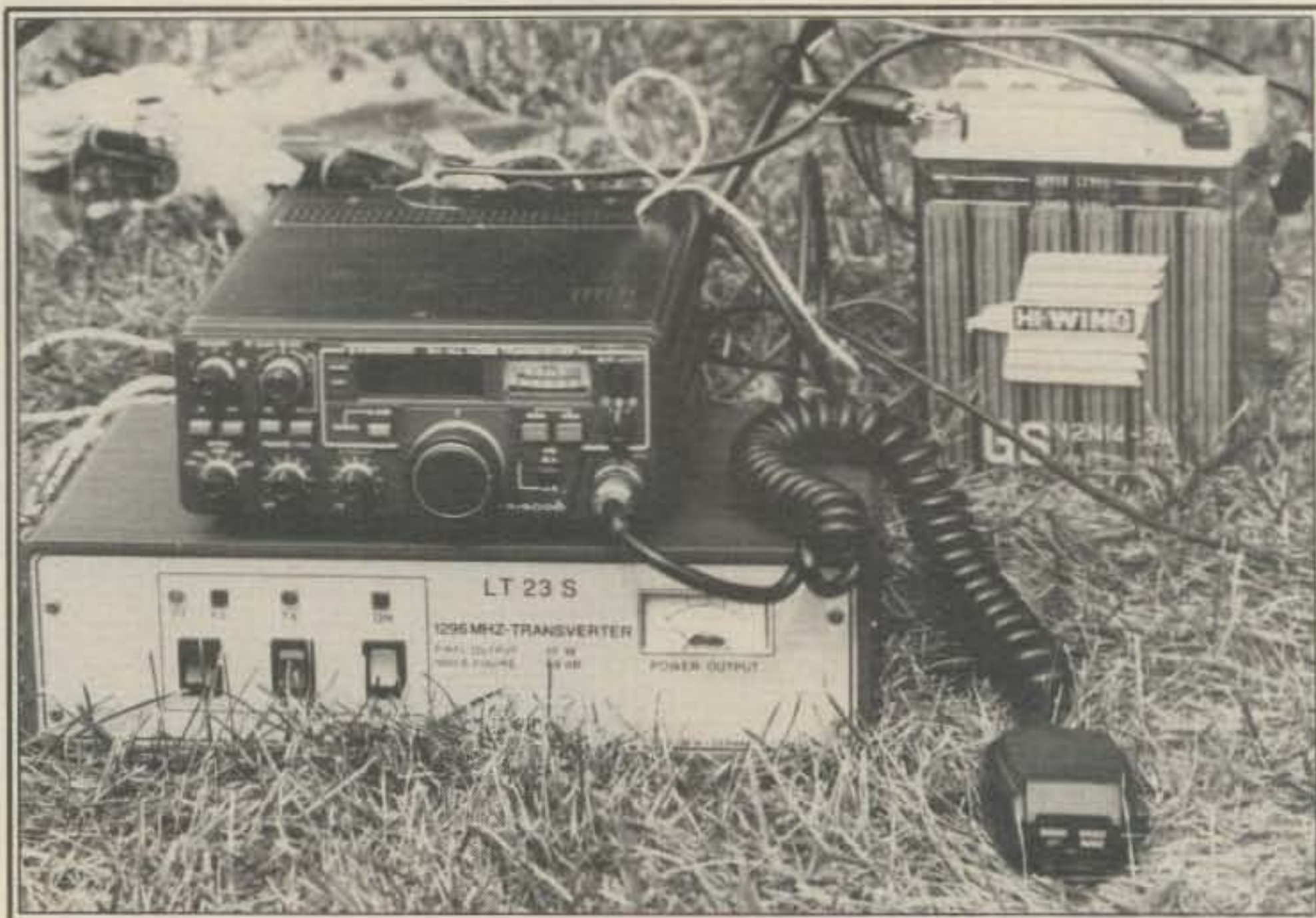
The 23 cm 10 watt transmitting equipment used for antenna gain testing at WB2WIK.
