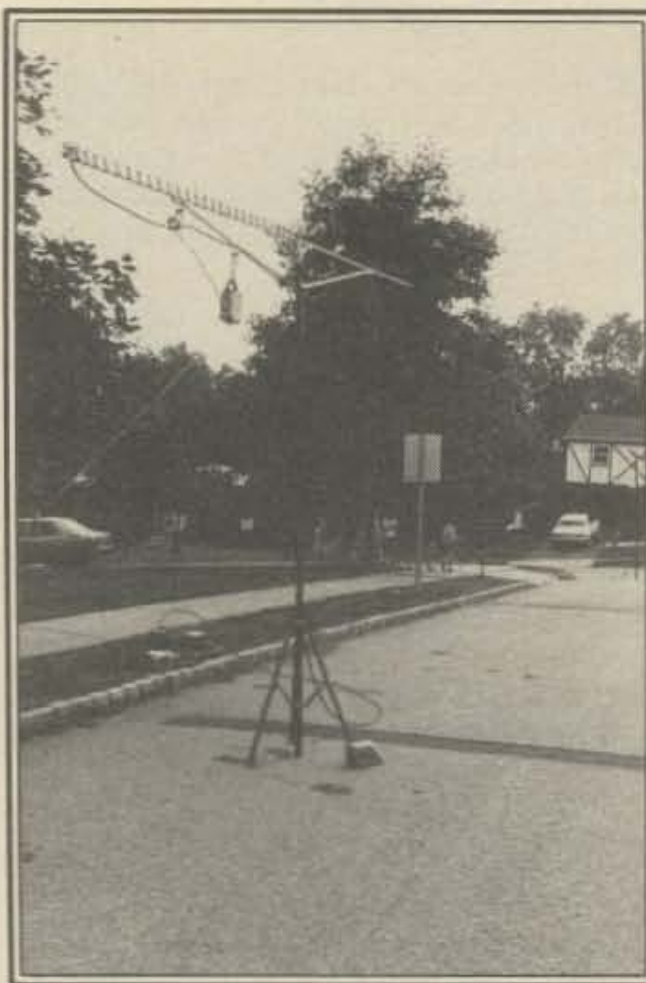
One end of the "antenna range," showing the "transmit" antenna on its 10 foot mast. The tree that looks close by isn't. It's about 30 feet to the side.
