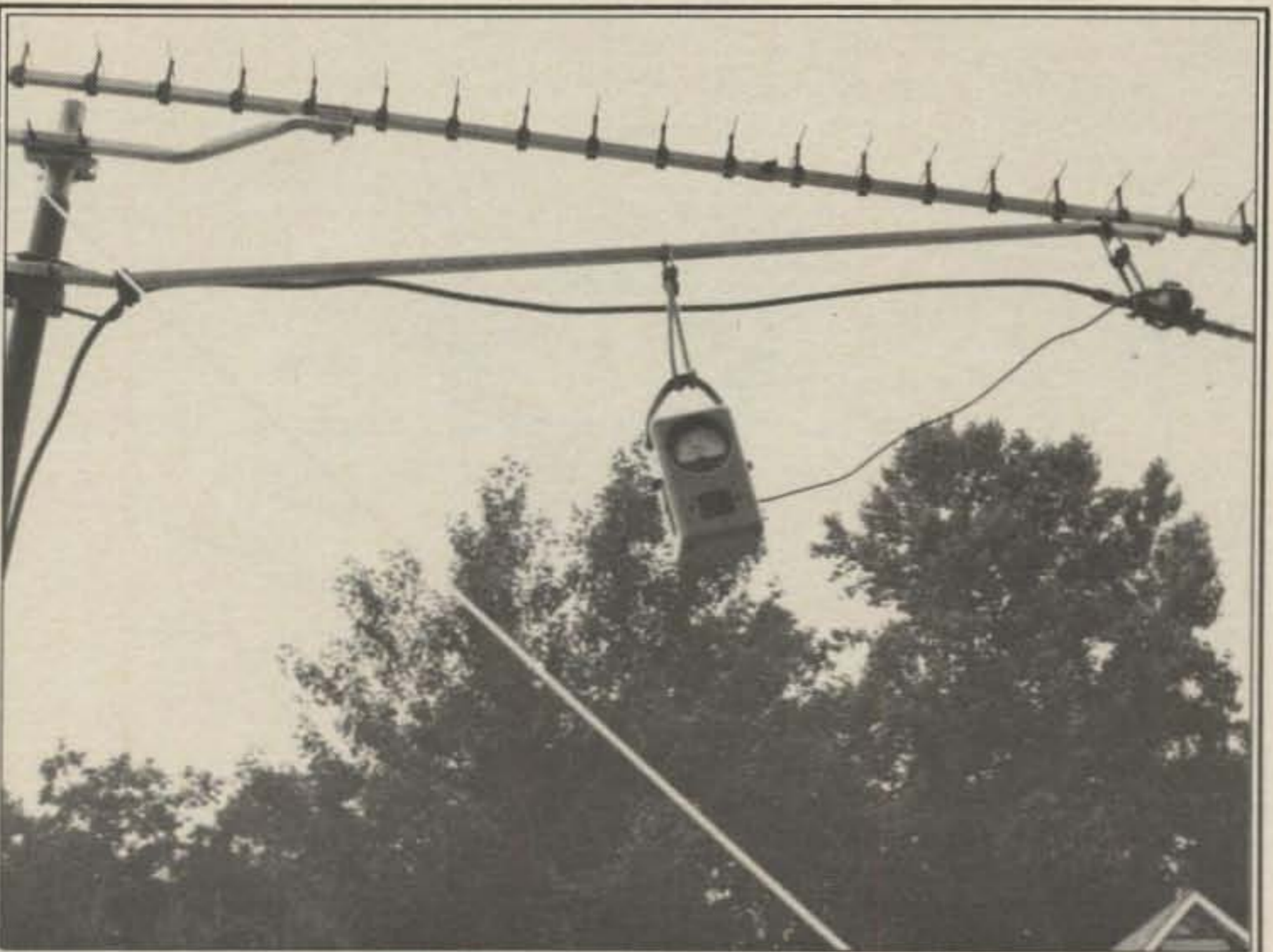
Bird Thru-line wattmeter hanging below the boom of the "transmit" 55-element Yagi. Its RF coupler is up by the boom, just inches from the driven element.
