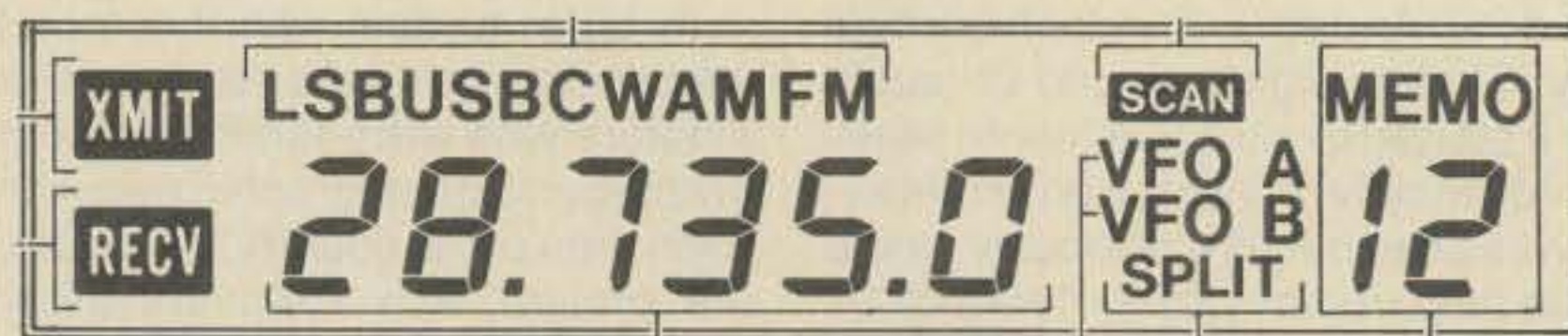
Fig. 1—Example of the ICOM's multifunction display. Each parameter appears as commanded by the rig's controls.
