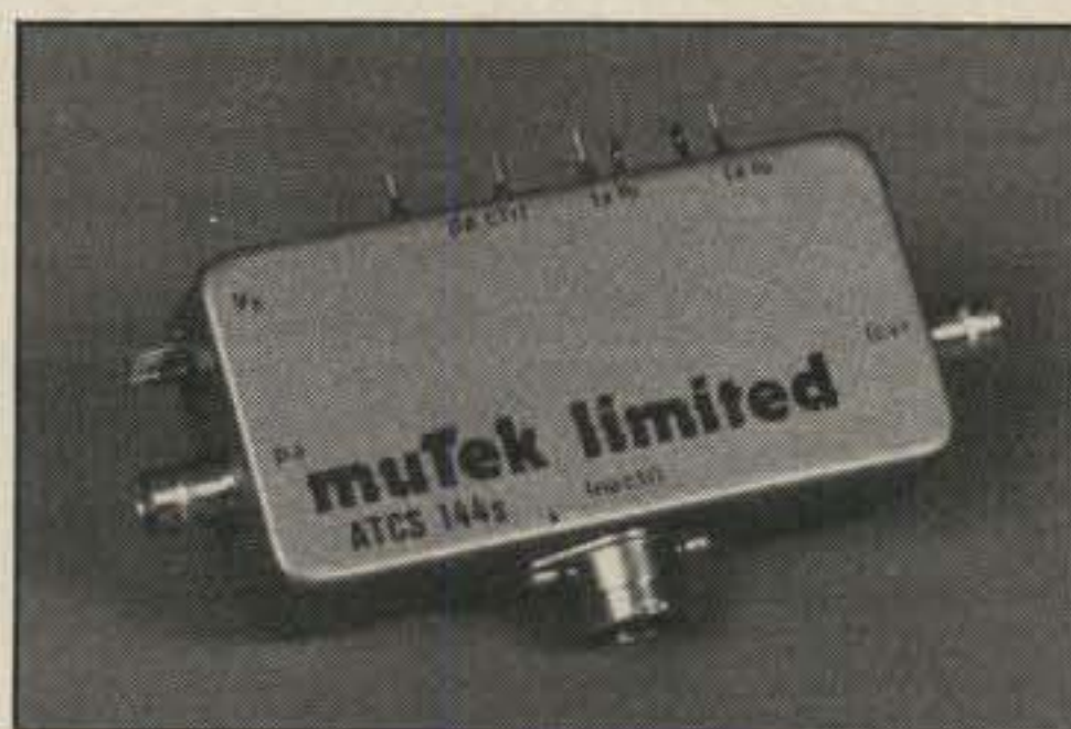
The muTek ATCS144S sequencing controller. DC and keying lines connect to feedthroughs while the exciter RF path is routed through the unit. Photo by KT2B.
