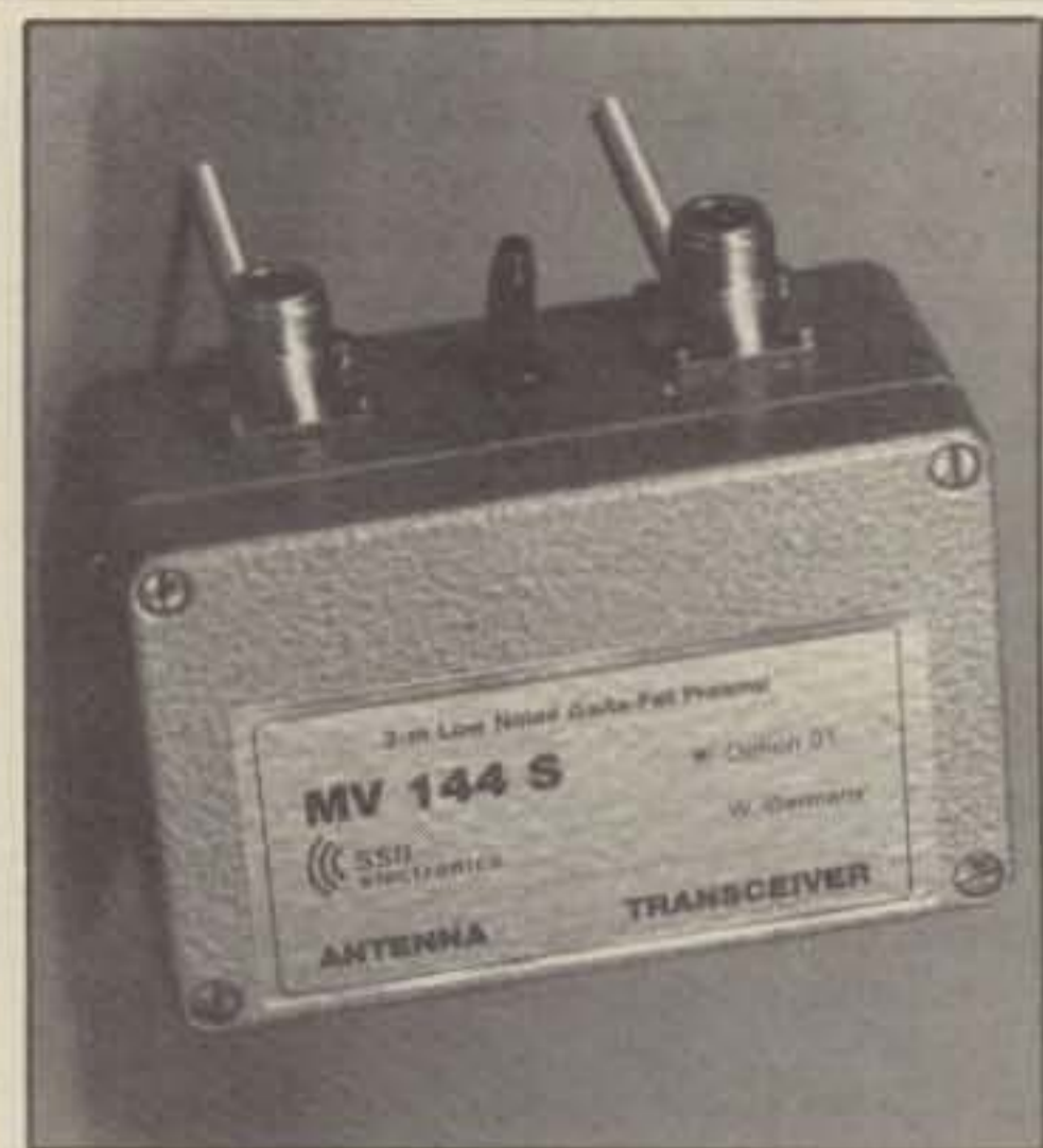
The SSB Electronic MV144S masthead preamp. RF connections are type N receptacles, and no additional connections are required. Photo by KT2B.
