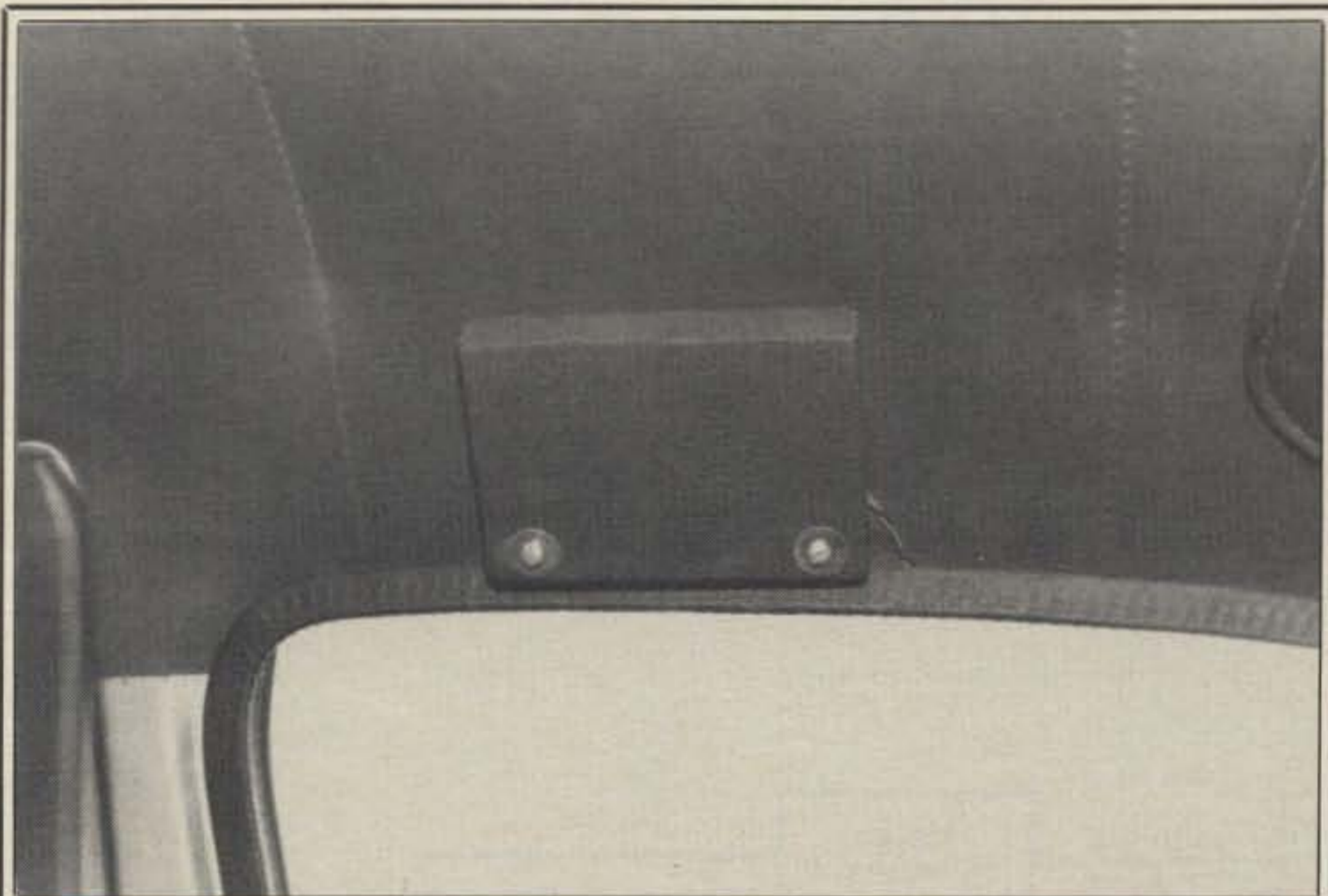
The mobile speaker installed in my Chevette. The unit measures 5" x 3 1/2" x 3/4" and doesn't interfere with the head room. Note the speaker cable tucked in behind the door trim.
