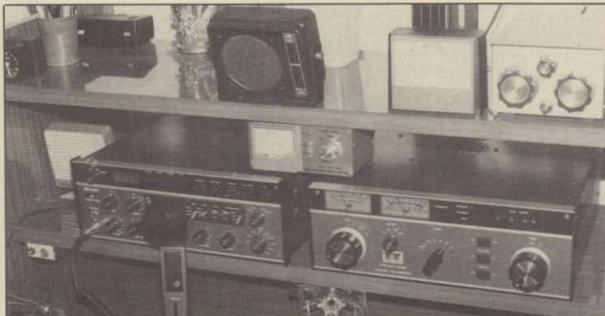
Photo 1. The Titan in operation next to a Corsair transceiver. It's hard to imagine a 3 kw linear almost the same size as its matching transceiver.
