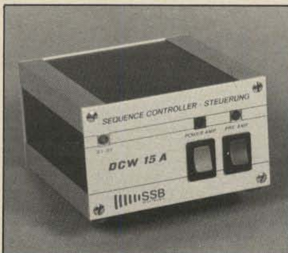
The sequencing controller model DCW15A by SSB Electronic is a handsome unit with rubber feet and panel LED status indicators. The RF transmission line is routed directly through this box, as well as through the masthead unit. Photo by KT2B.
