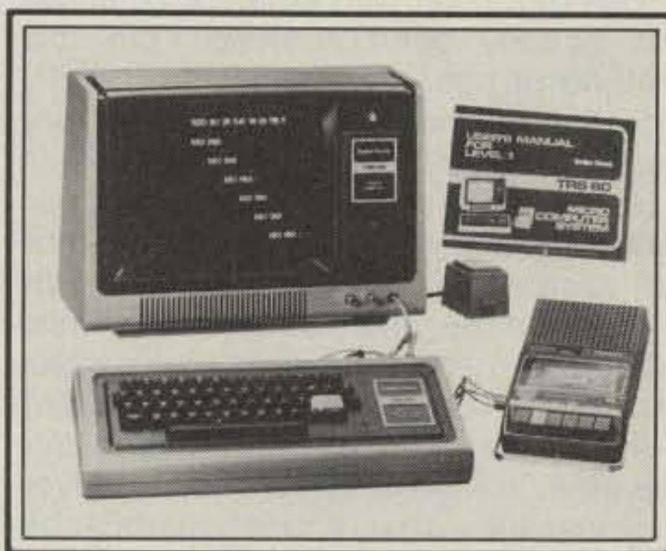
At least one firm has developed software to enable the Radio Shack Model I (shown here), III, and IV microcomputers to function as terminal node controllers (TNCs) for packet reception and transmission. (Photo courtesy Radio Shack)
