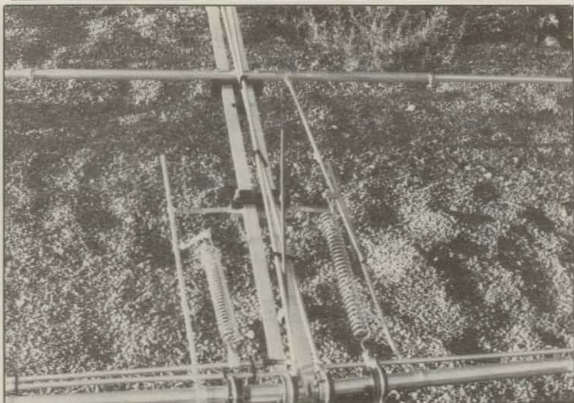
This is the rear of the antenna and on the right the 40 meter loading coil for the back element. At the left is the 30 meter arrangement.
