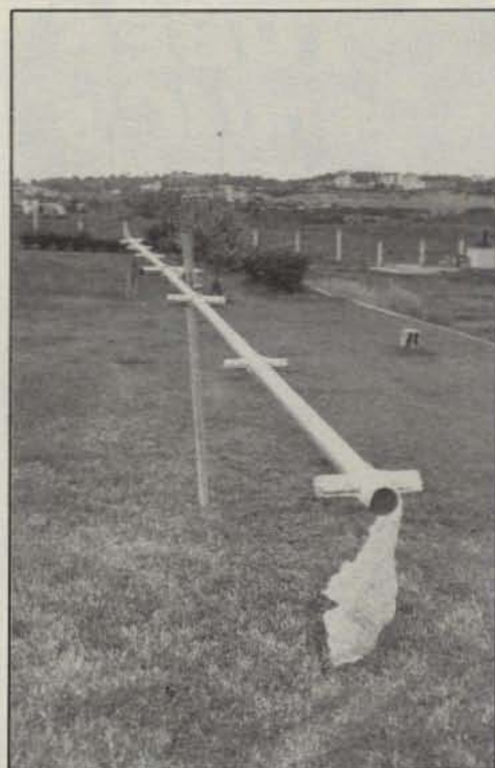
The TH7 was assembled on a temporary mast. Just the boom is shown on the mast.
