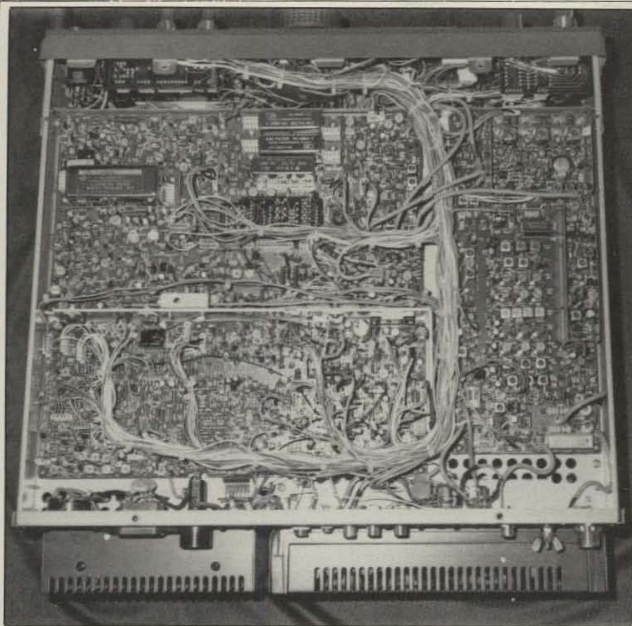
Taking off the bottom cover one sees a jungle of parts and wires. However, it is a very well-organized and well-labeled "jungle" in case you need to trace around it. Various of the optional IF filters are shown installed on the IF Unit board (upper left).
