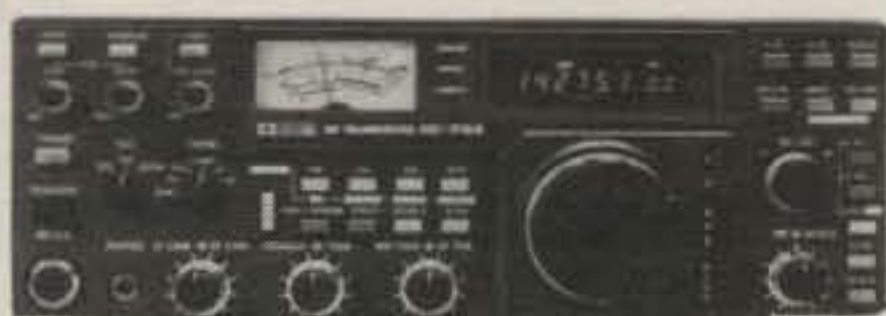
IC-751 9 band XCVR, 1-30 MHz
